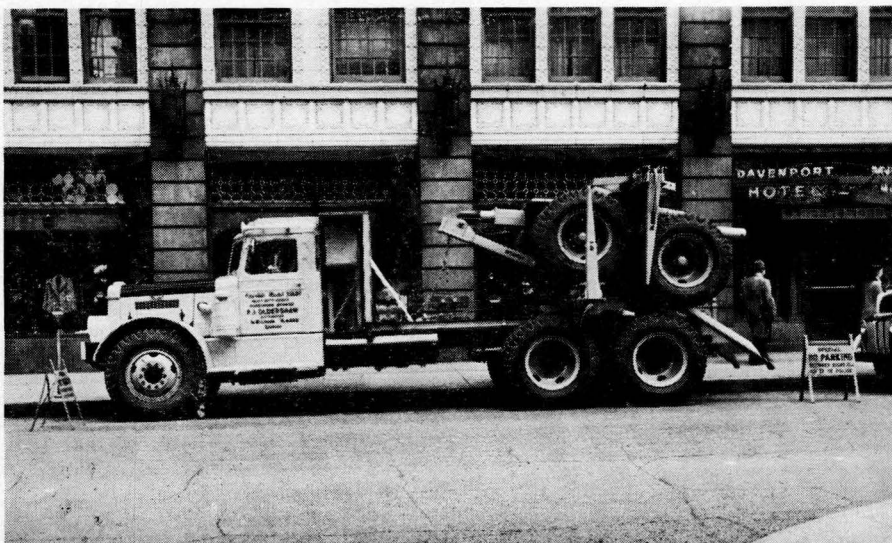
Peterbilt heavy duty logger, model 335 DT, with Fruehauf trailer, equipped with Hydro-tarder, displayed by P. J. Oldershaw, Spokane dealer.
