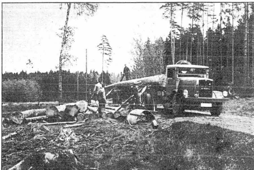
Motor truck logging is the common practice in the woods as it is in most regions of the United States. Power for the cross-haul loading is supplied by the truck engine. Tree lengths are commonly cut and hauled because of lower handling and transportation costs. These are cross-cut at the mills to suitable lengths to supply the local demand.
