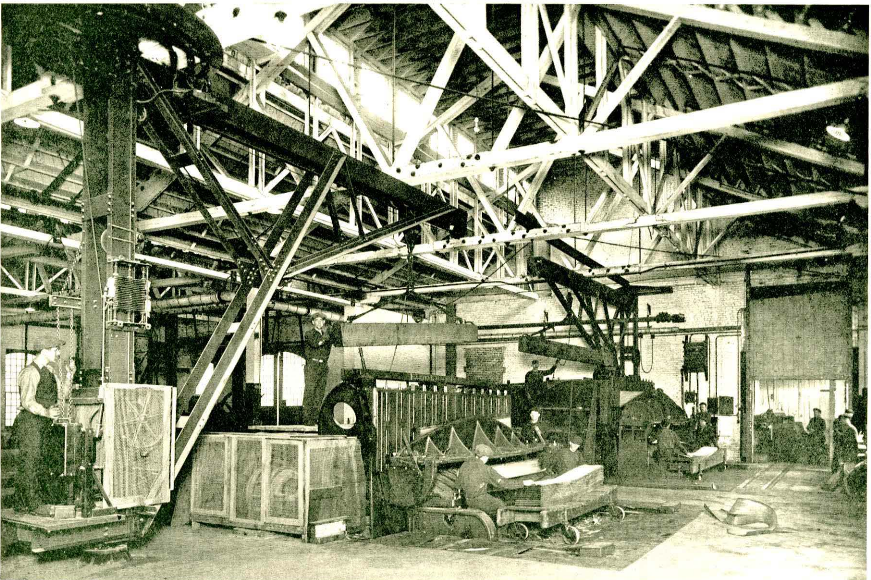
VENEER "SLICERS"—THE LARGER MACHINE ( nearest the wall ) IS OF OUR OWN DESIGN AND BUILT OVER 20 YEARS AGO. THE KNIFE IS 17 FEET LONG. TWO SEPARATE "BEDS" INTERCHANGEABLE, OBTAINES LOSS OF USE OF THE MACHINE WHILE "GRINDING" KNIVES, AND MAKES THIS MACHINE THE LARGEST PRODUCER IN THE WORLD. IT HAS CUT MANY MILLIONS OF FEET OF FINE FIGURED VENEERS, AND IS IN CONTINUOUS OPERATION.
