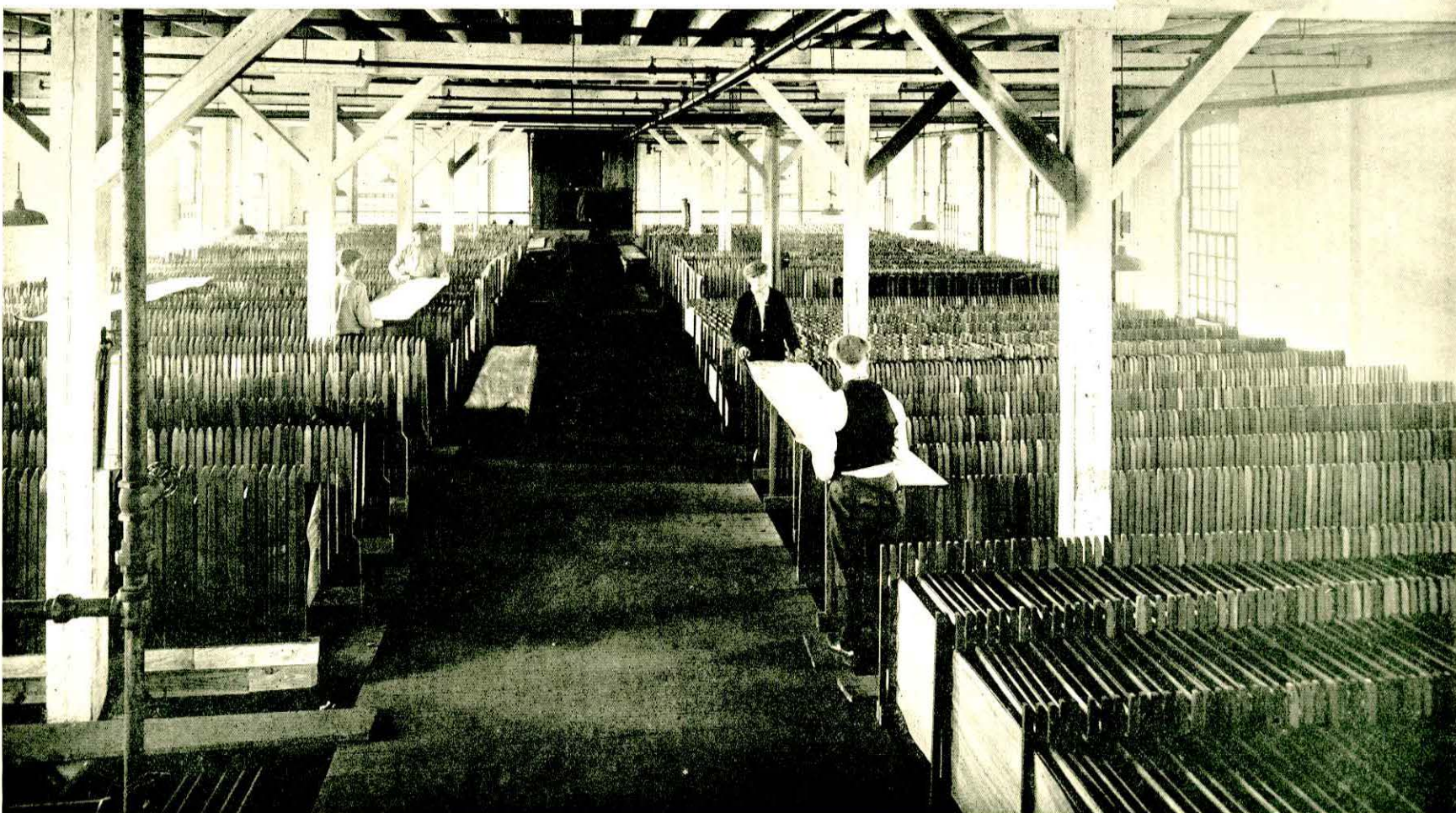
Top —AUTOMATIC VENEER DRYER—UNLOADING OR "DRY" END SHOWN. Lower —HEAT AND HUMIDITY CONTROLLED VENEER DRYING ROOM.
