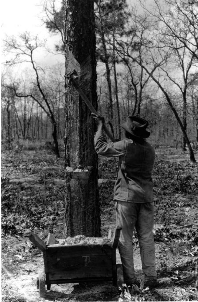
A worker in Florida scrapes hardened resin from a tree. The catface is visible at top. The photo is from "A Pictorial Album of the Naval-Stores Industry," published by the U.S. Forest Service in 1937. (FHS2024)
