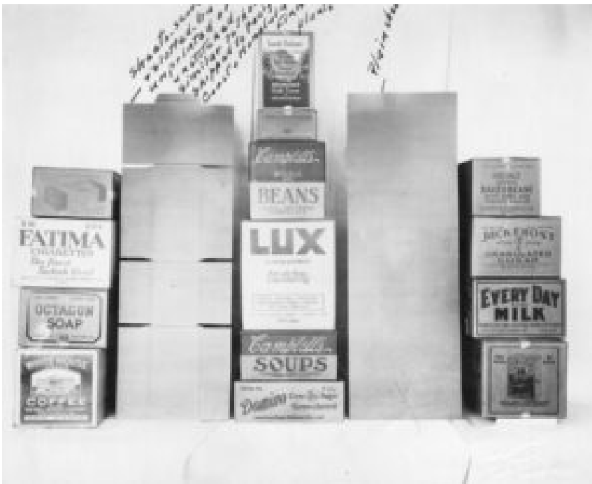
Printed finished boxes, plain box sheets, and sheets scored and slotted, but unprinted or unstitched similar to those shipped to finishing plants.
