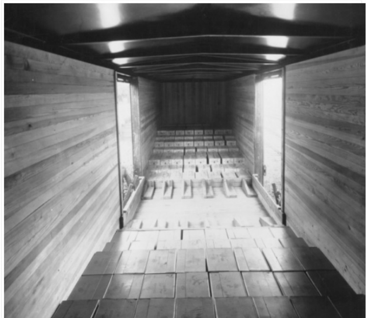
Testing for dynamite container shifting in box car. Wooden containers used on far end and solid fiber on the other.
