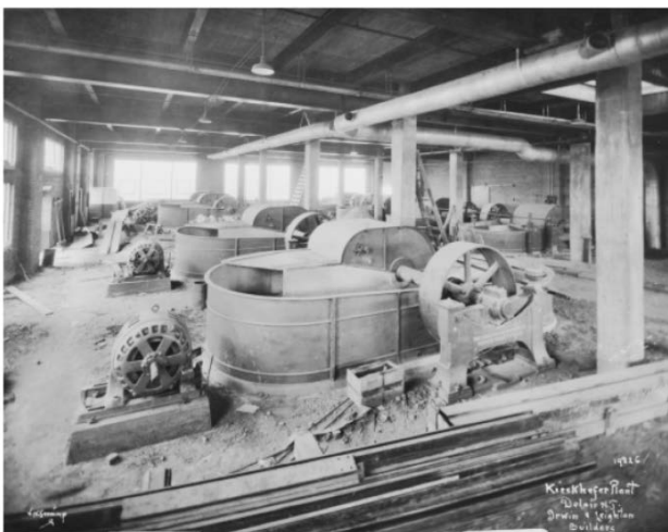
Noble and Wood (Hoosick Falls, NY) beaters. These machines were used to create containerboard pulp by breaking down wood fibers. The pulp would then be formed into sheets.
