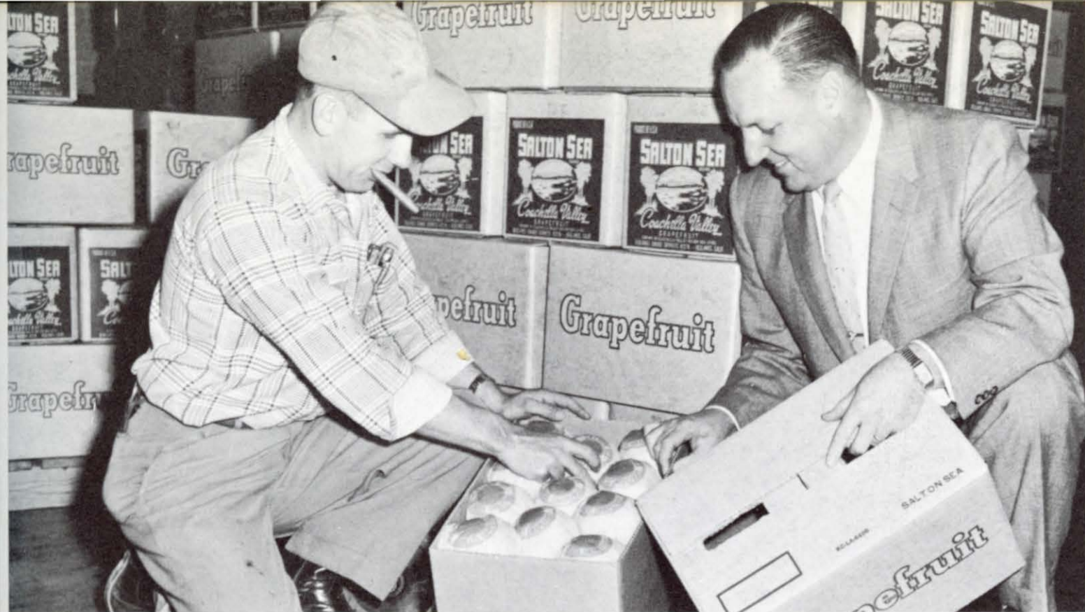
NEW 2-piece telescoping containers make fruit inspection easy for the buyer, provide double strength walls to permit higher stacking.
