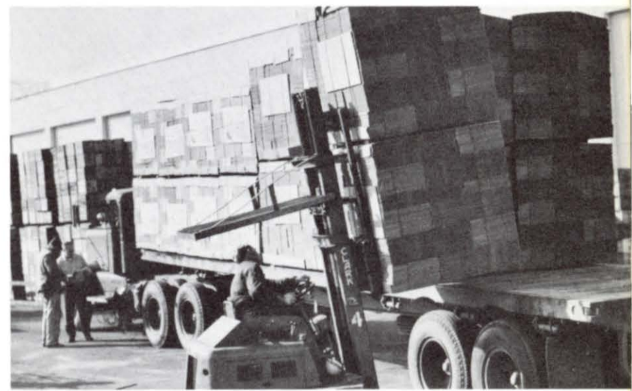
FRUIT BOXES arrive at packing plant in unit loads for efficient handling. Here, 1,500 boxes are being moved in one simple operation.
