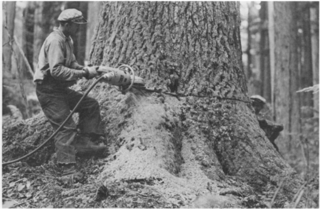
Later experiments included the cumbersome Wade drag saw, ca. 1930, which was a gasoline-powered rig used to buck logs. Since it pushed a crosscut blade back and forth, it shared little in concept with the chain saw at right, which was described in 1943 as an "electric tree felling machine." Drawing power from a portable generator, this saw permitted two loggers of the St. Paul and Tacoma Lumber Company to drop a mature noble fir in twelve minutes.
