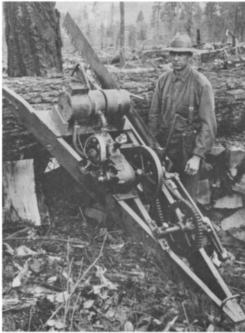
Later experiments included the cumbersome Wade drag saw, ca. 1930, which was a gasoline-powered rig used to buck logs. Since it pushed a crosscut blade back and forth, it shared little in concept with the chain saw at right, which was described in 1943 as an "electric tree felling machine." Drawing power from a portable generator, this saw permitted two loggers of the St. Paul and Tacoma Lumber Company to drop a mature noble fir in twelve minutes.
