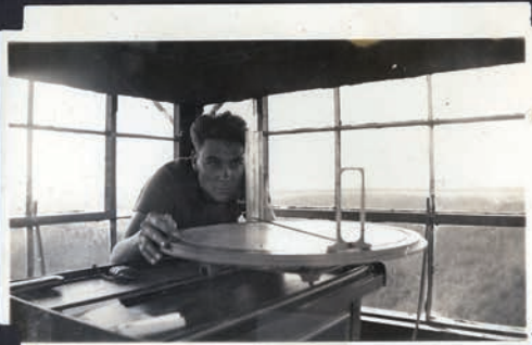
Homer Peters was putting the "bead" on a smoke spotted from the Red Bridge tower. After sighting thru this Osborne fire finder and getting a line on the smoke a degree reading is taken and called in to the Guard Station. The degree readings on our maps correspond with those in the towers and that way we get the location of the fire.
