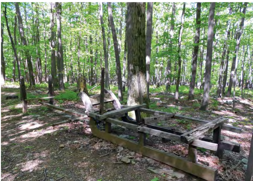
Using a pair of mules or horses, wood haulers moved half a cord on sleds like this to a charcoal hearth. They would unload the wood on both sides of the sled around the hearth, then return for another load.
