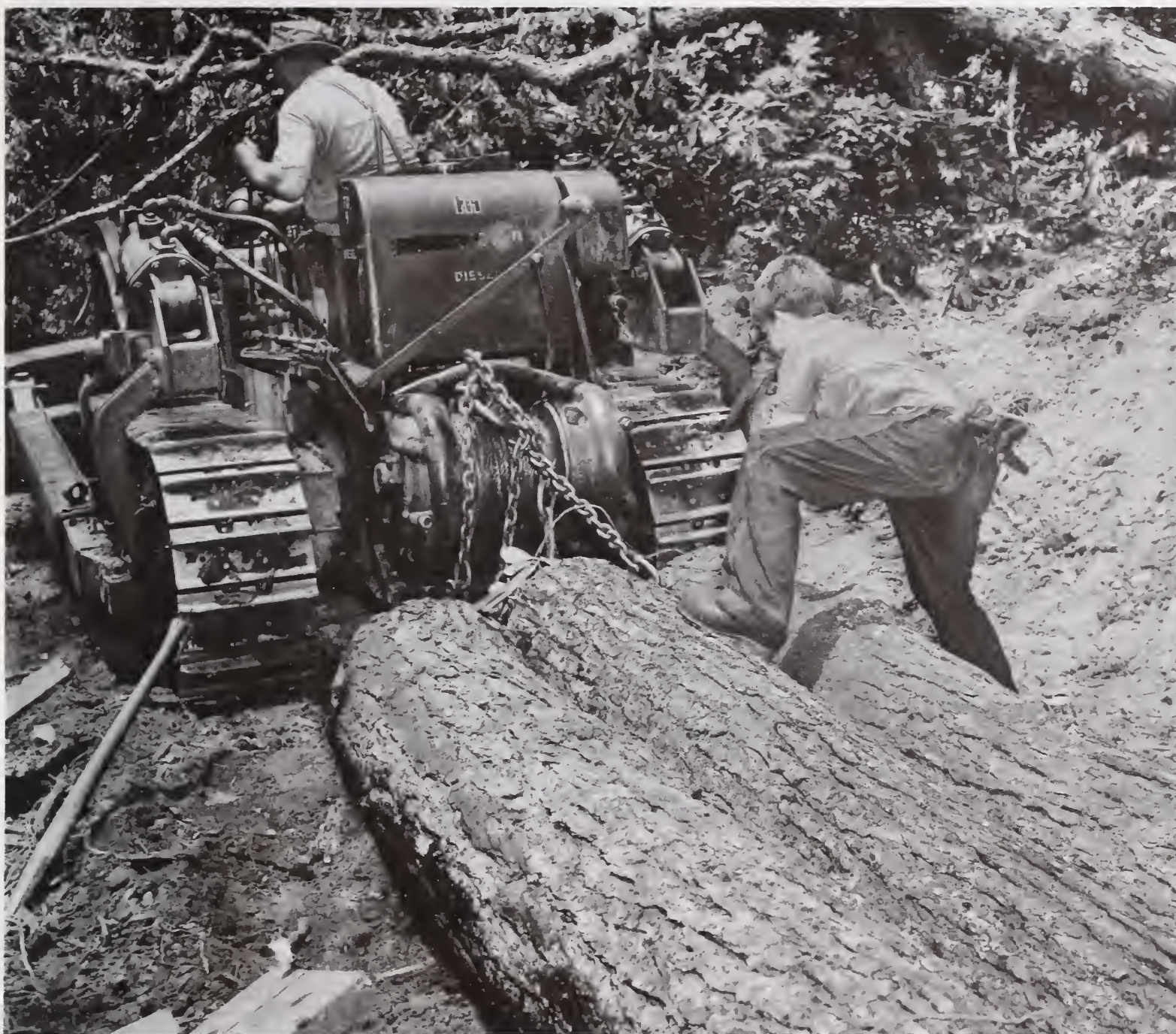
Figure 97.—Skidding hemlock logs to landing by tractor and winch on Reed Creek timber sale in Bear Hollow, Wythe Ranger District, Jefferson National Forest, southwestern Virginia, in July 1955. (Forest Service photo F-479067)
