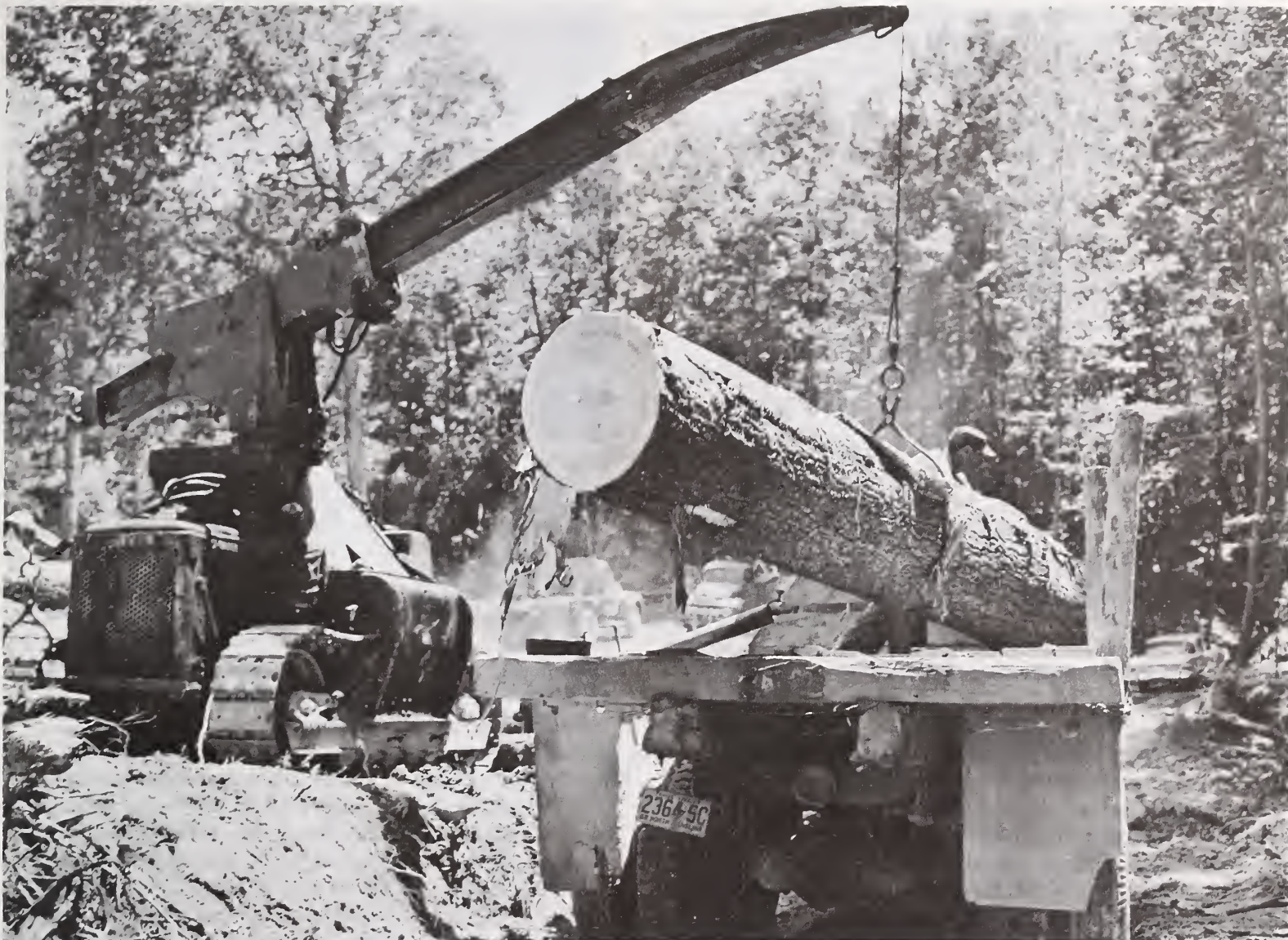
Figure 109.—Tractor-mounted power loader dropping a big white pine sawlog onto a truck at a Forest Service timber sale in Hurricane Gap section of Nolichucky Ranger District, Cherokee National Forest on the Tennessee-North Carolina State line adjoining Hot Springs Ranger District of Pisgah National Forest, in May 1962. (Forest Service photo F-502185)
