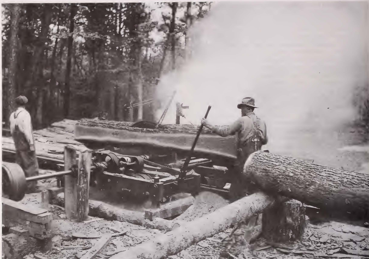
Figure 43.—Portable sawmill with circular saw powered by oil distillate, cutting white oak log. Laurel Lumber & Stave Company, Daniel Boone (then Cumberland) National Forest, Ky., August 1937. Smoke came from a burning pile of slabs. (NA:95G-365412)
