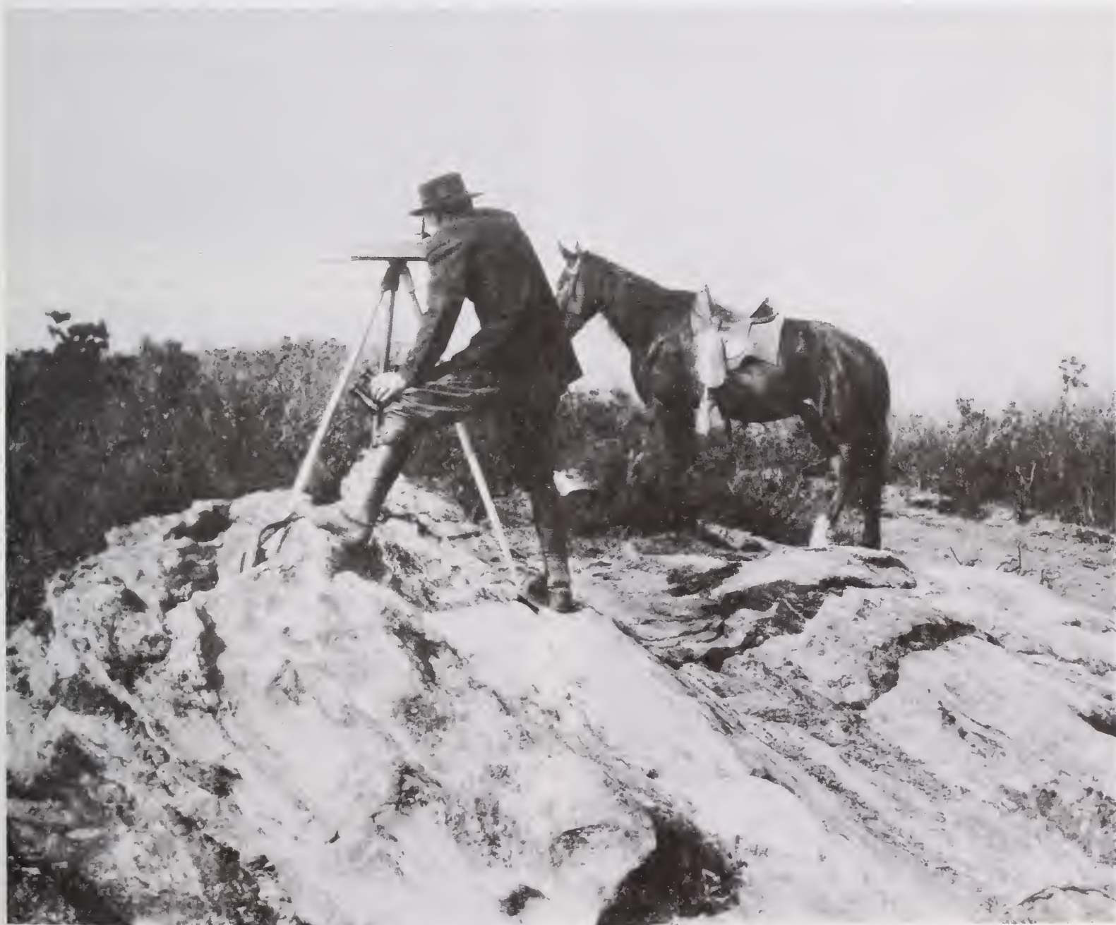
Figure 33.—Forest Service ranger on top of Satulah Mountain near Highlands, N.C., using an alidade to locate on his map a forest fire to the northeast in the direction of Chimney Top Mountain on the old Savannah Purchase Unit in April 1916. Note binoculars. This area near South Carolina and Georgia became part of the Nantahala National Forest in January 1920. (NA:95G-27296A)
