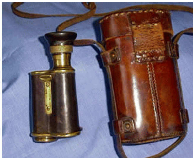
Early 20th century leather covered brass monocular by CPGoerz with original leather case. This item was only produced between 1898-1911.
