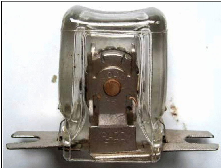
Old telephone lightning arrester made of clear glass whith what looks like a mica bottom.
