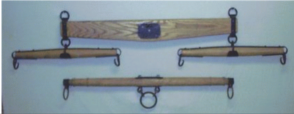
Wagon hitching equipment: double tree on the top and single tree below.
