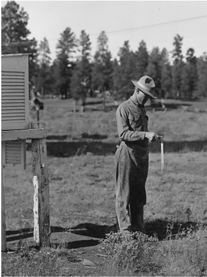
Gus Pearson reading a sling psychrometer at a Fort Valley meteorological station in 1910.
