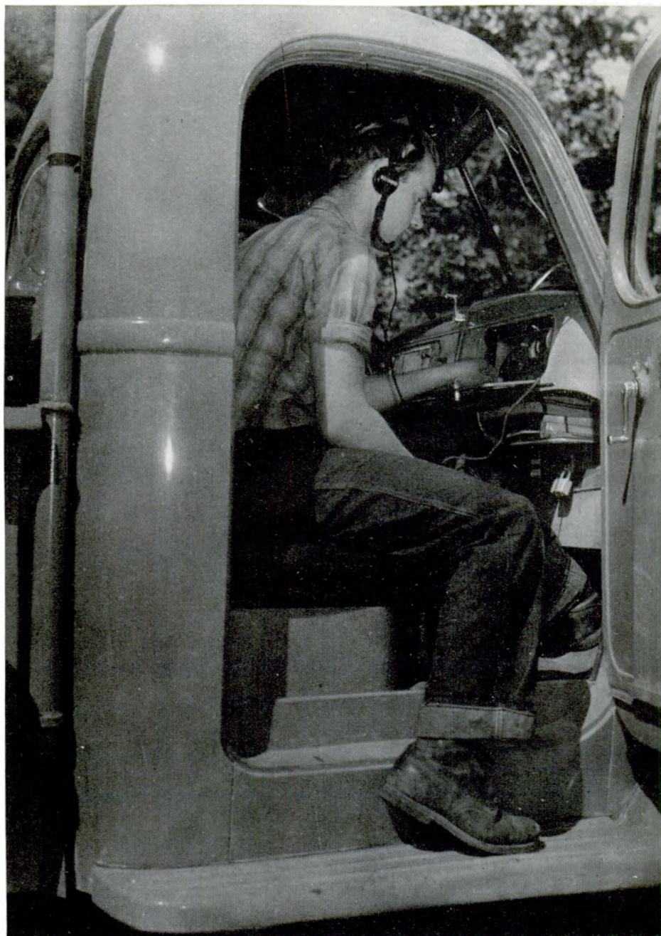
Radio set installed in the glove compartment of a small fire truck with an outside aerial makes possible radio communication while the truck is en route to a forest fire.
