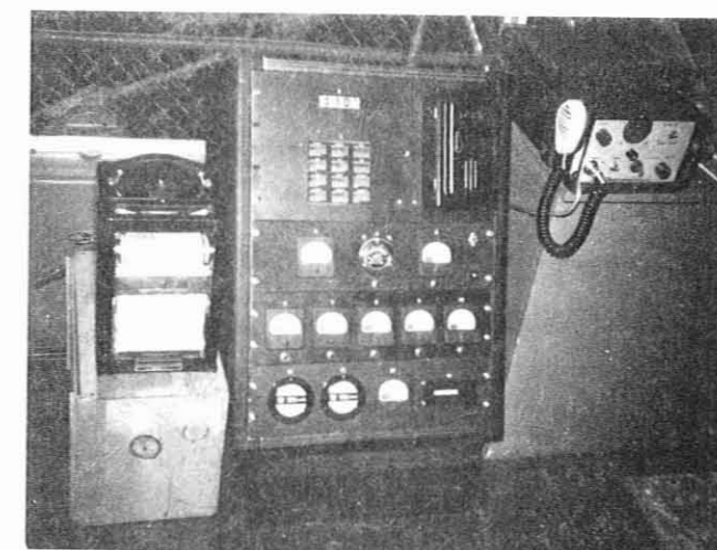
Figure 138. Instruments of the remote Forest Service radio relay repeater station powered by solar energy cells at a test installation in California. Developed by Guy Wood, shown left to right are strip chart recorder, special instrumentation, and the Motorola repeater unit. (Forest Service photo, History Section)
