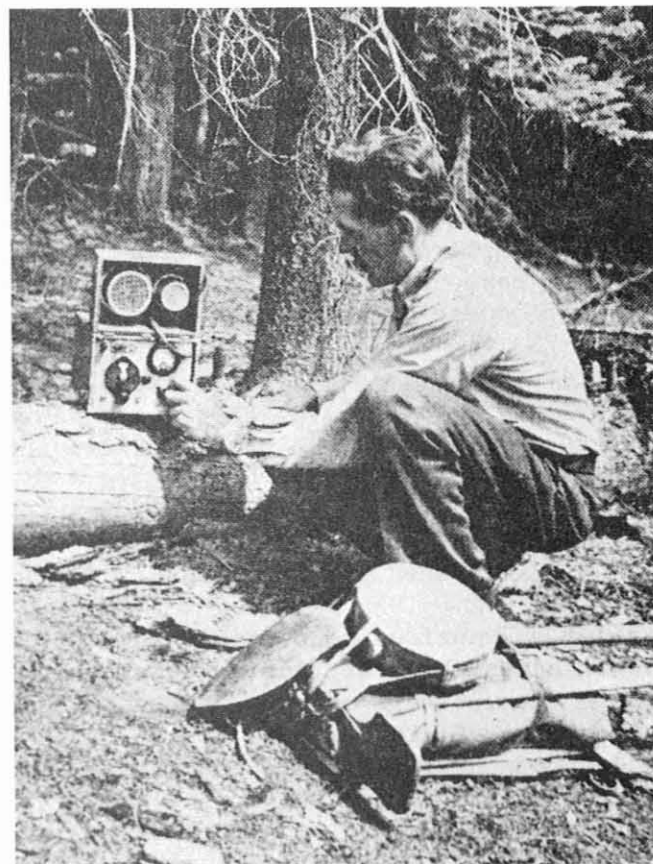
Figure 120. A fire scout with his lightweight SPF set. Note pulaski (grubhoe-axe firefighting tool), shovel, canteen, and bedroll in foreground. (Forest Service photo, History Section)
