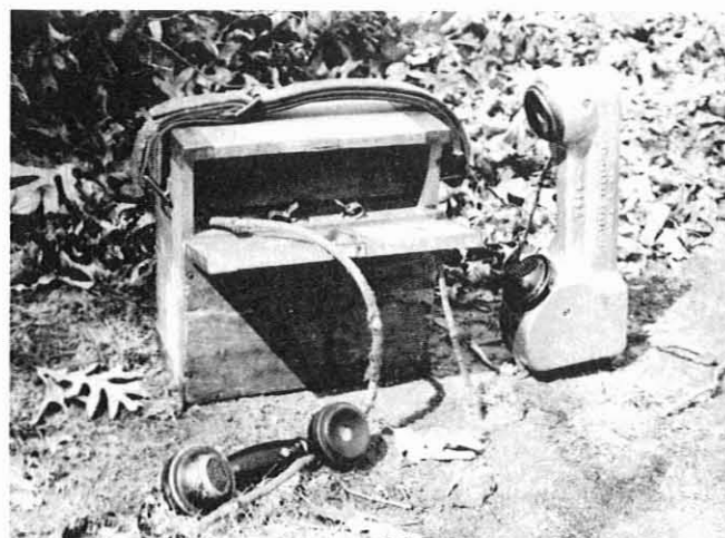
Figure 111. A strong emphasis on portability in communications began early on the National Forests. These Forest Service portable telephone handsets, made by Kellogg, were carried by Rangers and clamped to field telephone lines for use. Wooden box model (C-608) has a folding crank on the right side. The front is hinged to open down. This model, which dates from the late 1920's, was used through the 1930's. A more truly portable set in the modern sense, the aluminum model B-209 dates from the late 1930's and was used through the 1940's. It has an external contact for the telephone wire and two buttons to press--one to send a sound to alert the other party on the line, and one to press while talking. (Forest Service photo, History Section)
