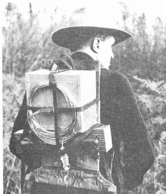
Figure 50. Portability of the type P radio is demonstrated by Harold Lawson of the Radio Laboratory. Note antenna loading coil and battery under container. (Forest Service photo, History Section)
