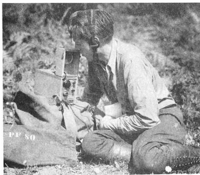
Figure 43. Demonstration of the type PF voice radio set, developed in 1933 by Squibb and Lawson at the Radio Laboratory. (NA:95G-280931)
