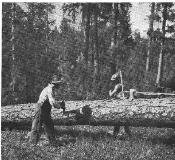
Bucking trees into logs. Note measuring stick, wedges, and sledge.
