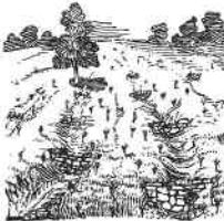
Check dams retard water movement.
