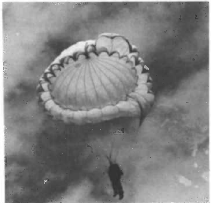
The 30 foot diameter Eagle parachute was the first canopy style used by the smokejumpers. Used until 1944.
