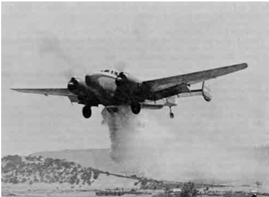
A PV-2 drops a load of water in a test run on the Medford Airport. The coverage is laid down in a pattern approximately 50 feet wide and 100 feet long.
