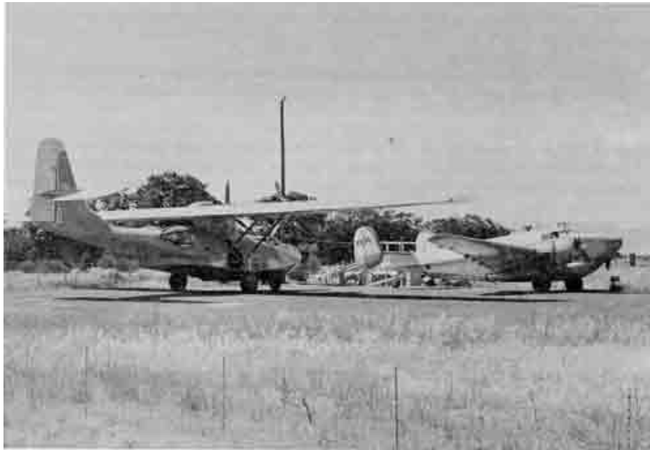
Two tanker planes from Rosenbalm Aviation wait on landing pad to be loaded with fire retardant. Each plane holds a 1000-gallon payload.
