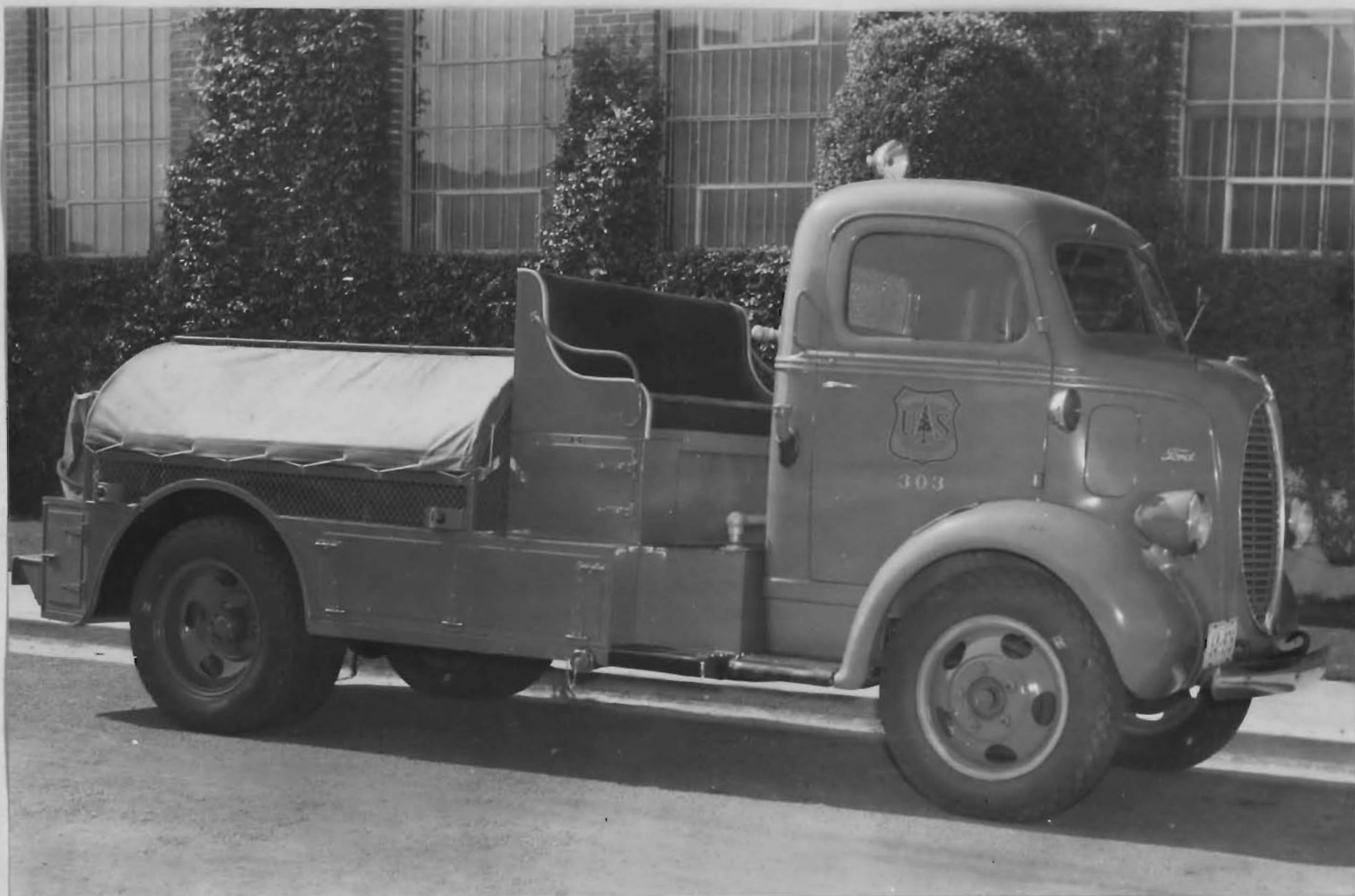
(Photo by U.S. Forest Service). 1940 Model Tank Truck (290 gals. capacity) on 2 Ton "Cab-over Engine" type of chassis. Note well balanced load on 134" wheel base - flush panel bodywork - California Region - U.S. Forest Service.
