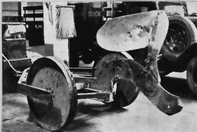
(Photo by U.S. Forest Service - Fire Equipment Handbook.) Fire Line Trencher used with tractor in fire suppression - Pacific North-West Region - U.S. Forest Service.
