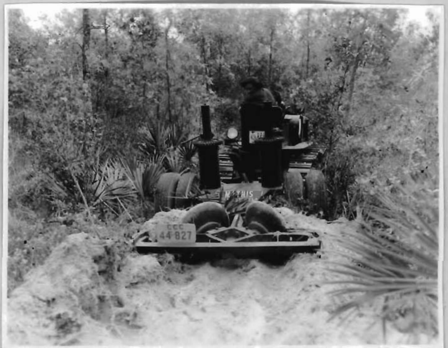
(Photo by U.S. Forest Service). Special two-disc fire line plough used on Florida National Forest - Florida.
