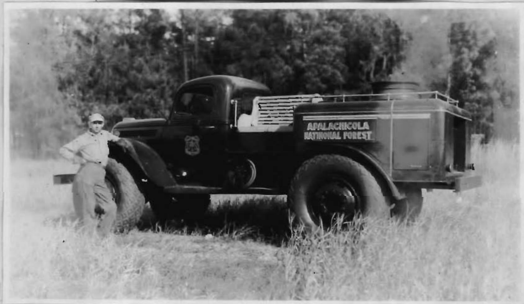
(Photos by U.S. Forest Service). Marsh Buggy - 4 wheel drive Marmon Harrington Ford developed for use as tank truck (Tank 425 gallons). Florida National Forest.
