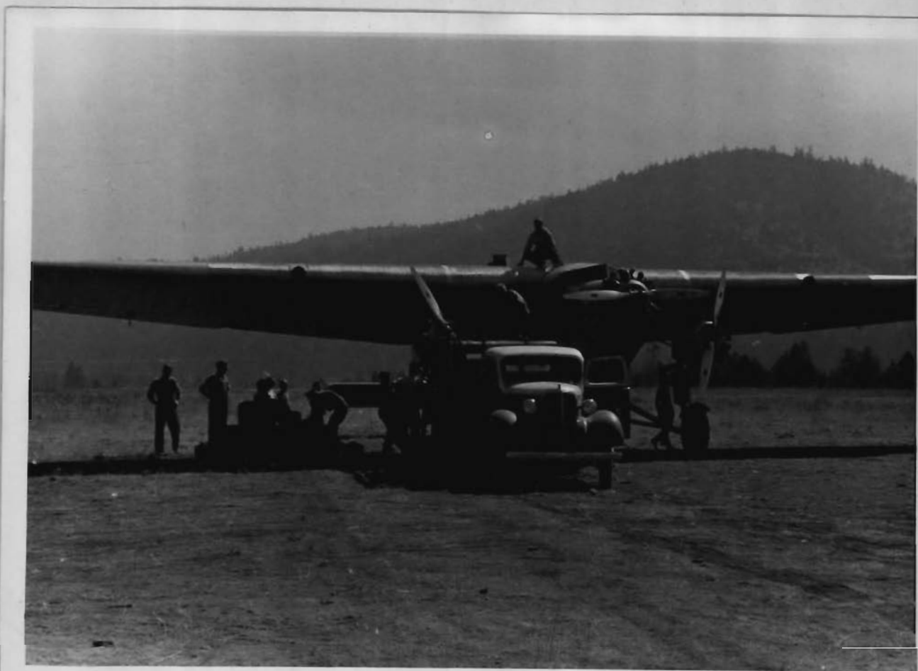
(Photo by K.D. Swan - Courtesy U.S. Forest Service). Loading fire equipment (4500 lbs. load) in Ford Tri-motor Plane McCall - Idaho.
