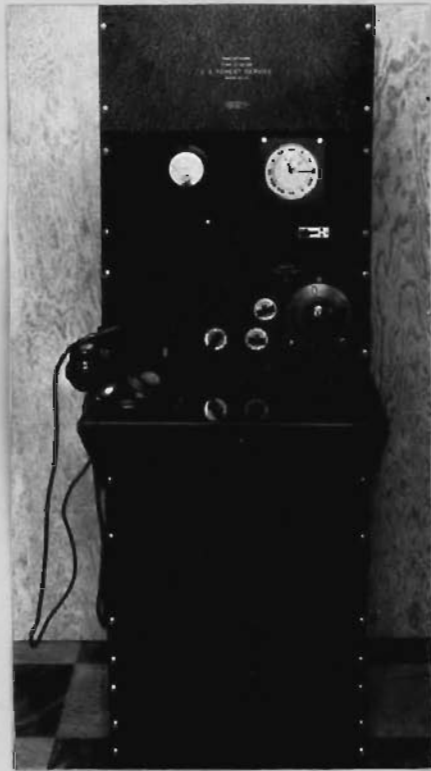
(Photo by U.S. Forest Service). Type U (U.H.F.) Radiophone used by U.S. Forest Service.
