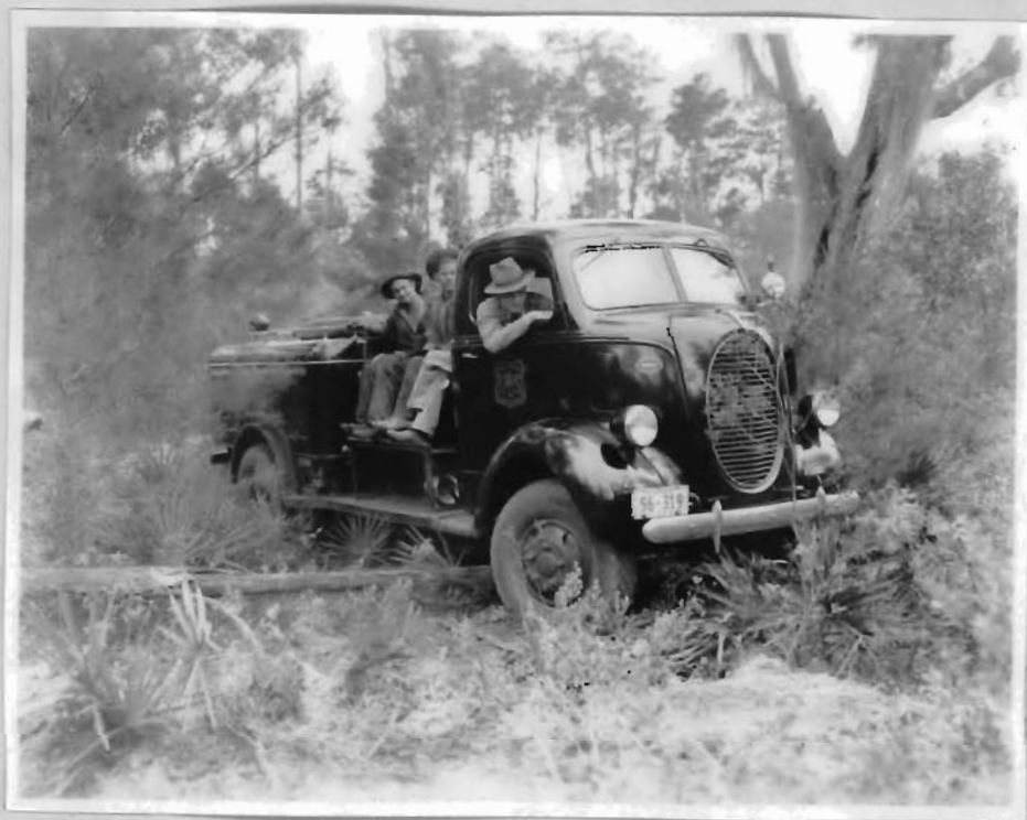
(Photo U.S. Forest Service). Marmon Harrington 4 Wheel Drive on "Cab-over Engine" 2 ton Ford Chassis, - developed as Tank Truck of 425 gal. capacity - Florida National Forest.
