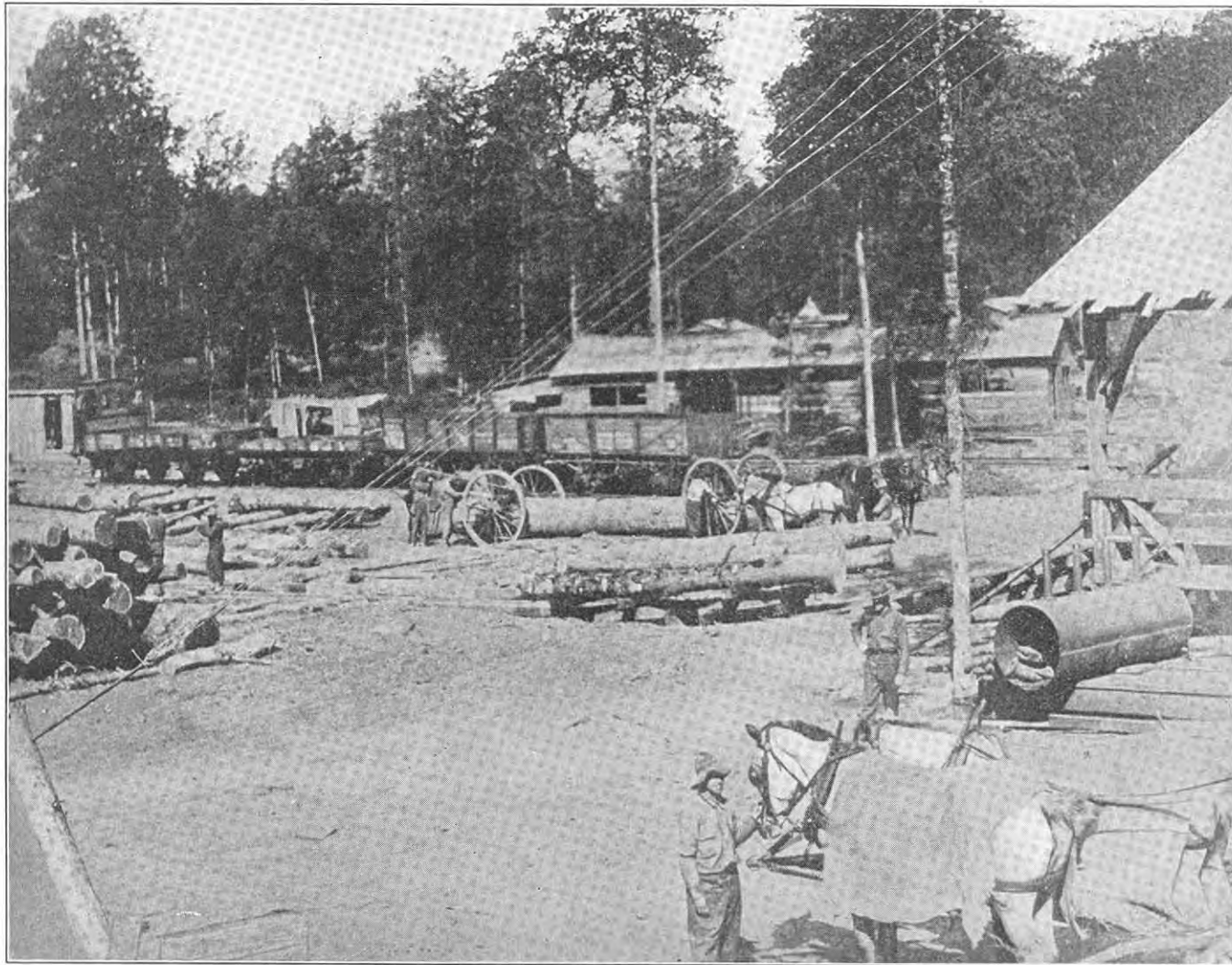
AMERICAN OPERATIONS IN PROGRESS IN A FRENCH HARDWOOD FOREST. IN THE CENTER A LOAD OF LOGS ON A CAR ON THE WAY UP THE INCLINE INTO THE MILL
