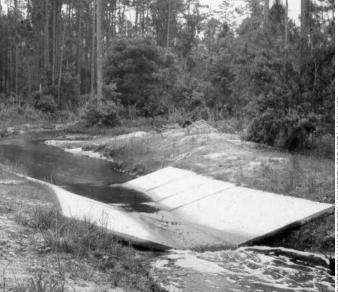
At the Bradford Forest in Florida, the Intensive Management Practices Assessment Center (IMPAC) Study addressed runoff and water quality for low-relief watersheds. Special control sections were necessary to gage runoff. In the heat of Florida, refrigerated storage was also used on site to preserve samples.
