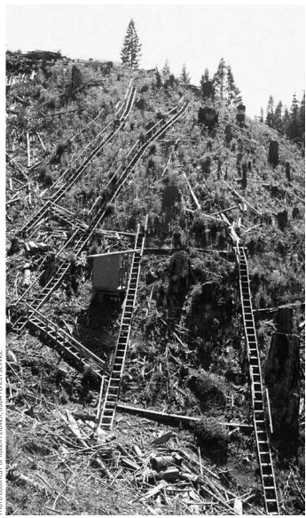
Process studies of soil moisture, subsurface flow, and pipeflow at Caspar Creek assisted in understanding effects of logging on streamflow and erosion. Summer 1991.
