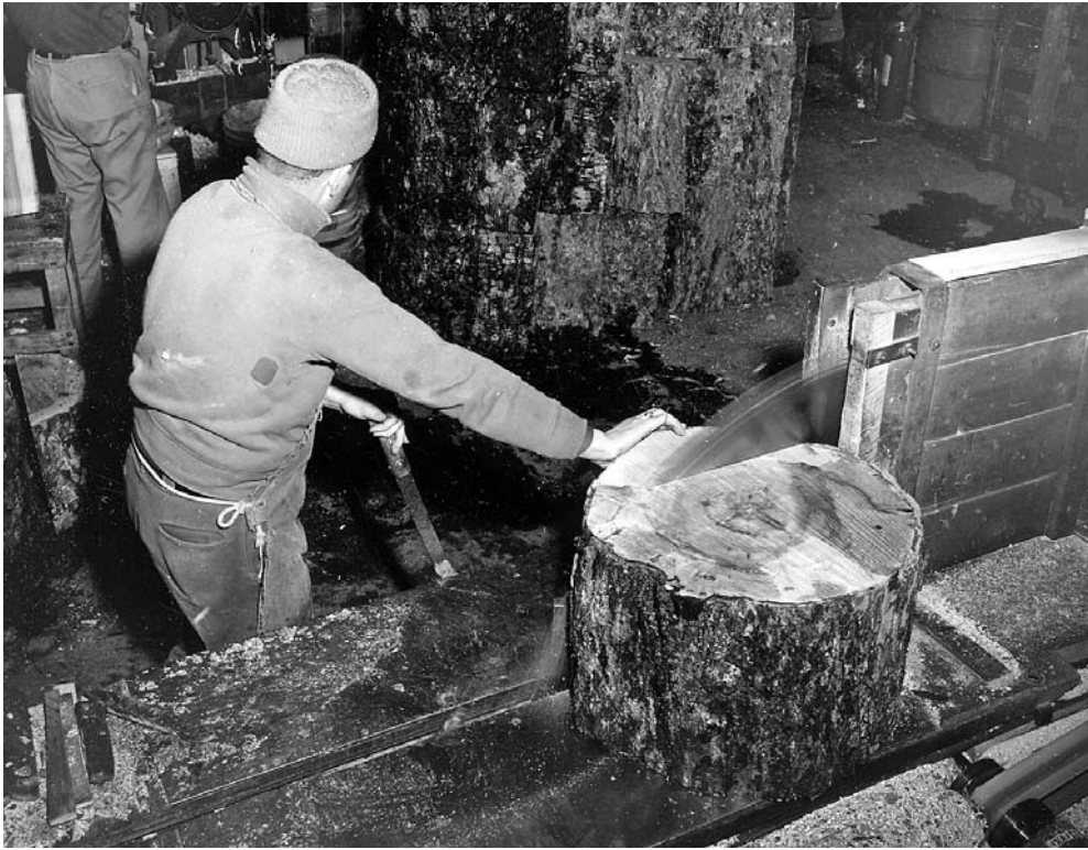
After logs are cut into bolts 18 to 22 inches in length on a bar saw, the bolts are then cut vertically into bowl blanks using a circular saw, creating one flat side opposite the rounded original exterior side. Photo dated February 1965.
