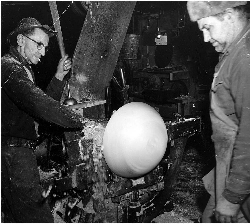
“Turning, outside already smoothed.” The flat bottoms on bowls were originally cut on the lathe and later sanded smooth.
