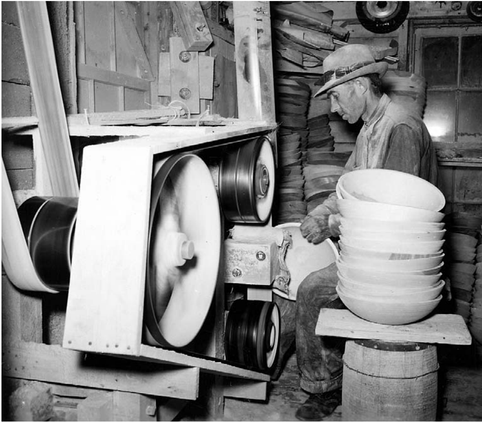
A Granville employee sands and smooths maple bowls, June 1941. After sanding, the bowls still needed to be dried and then sealed.
