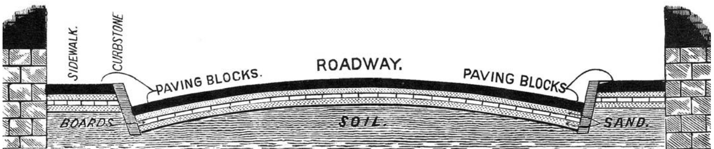
Samuel Nicholson’s patented paving technique quickly fell out of favor because he spaced the blocks too far apart and because “the foundation was usually of untreated planks, laid directly upon earth, so that they soon decayed, while the pavement sank into ruts and holes.” This cross section shows the plan used by the Hale Pavement Company of Staunton, Virginia, in the 1880s.
