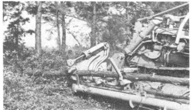
Shortwood stick being bucked and dropped in front of harvester. Toothed carriage moves stem forward 5'.
