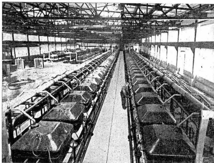
Hooker Cells in the Electrolytic Bleach Plant
