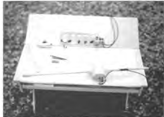
Figure 10: Hand instruments used with the proton magnetometer investigations at Angel Mounds. The long device is a probe that was connected to a receiver to transmit signals from the soil to detect prehistoric houses, pits, and other anomalies buried below the ground surface.
