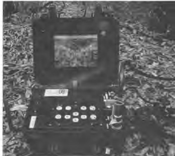
Figure 12: Close-up of ground penetrating radar instrument (GPR) with display of anomalies identified by the readings. This equipment was used during investigations at Indian Cave by Ball State University in 1997.
