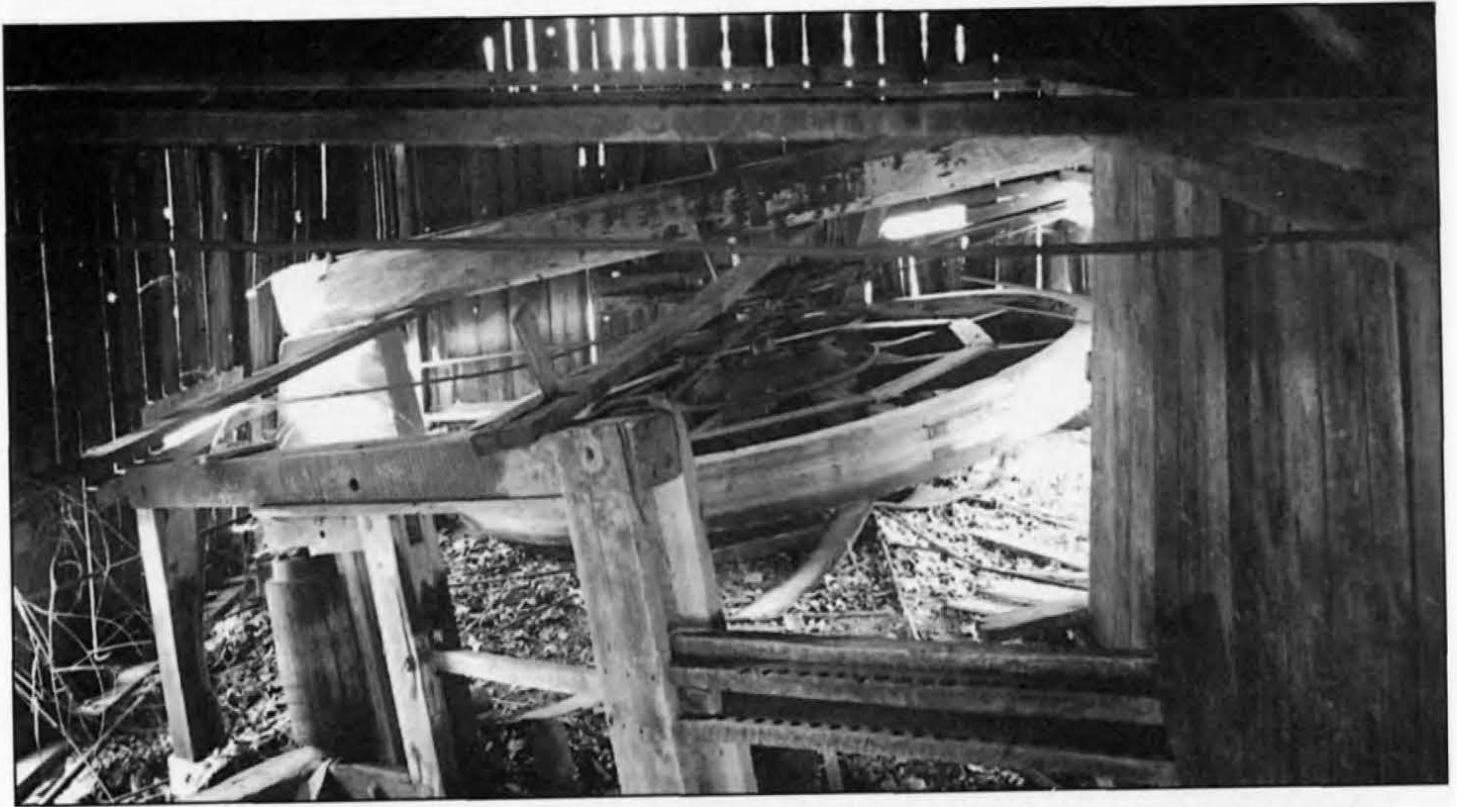
Wooden bandwheel double-eccentric power, Lot 202. Tiona Field, 1994. The bandwheel is installed parallel to the slope of the hill. The sash-mounted belt tensioner in the foreground is a very old example. Phil Ross
