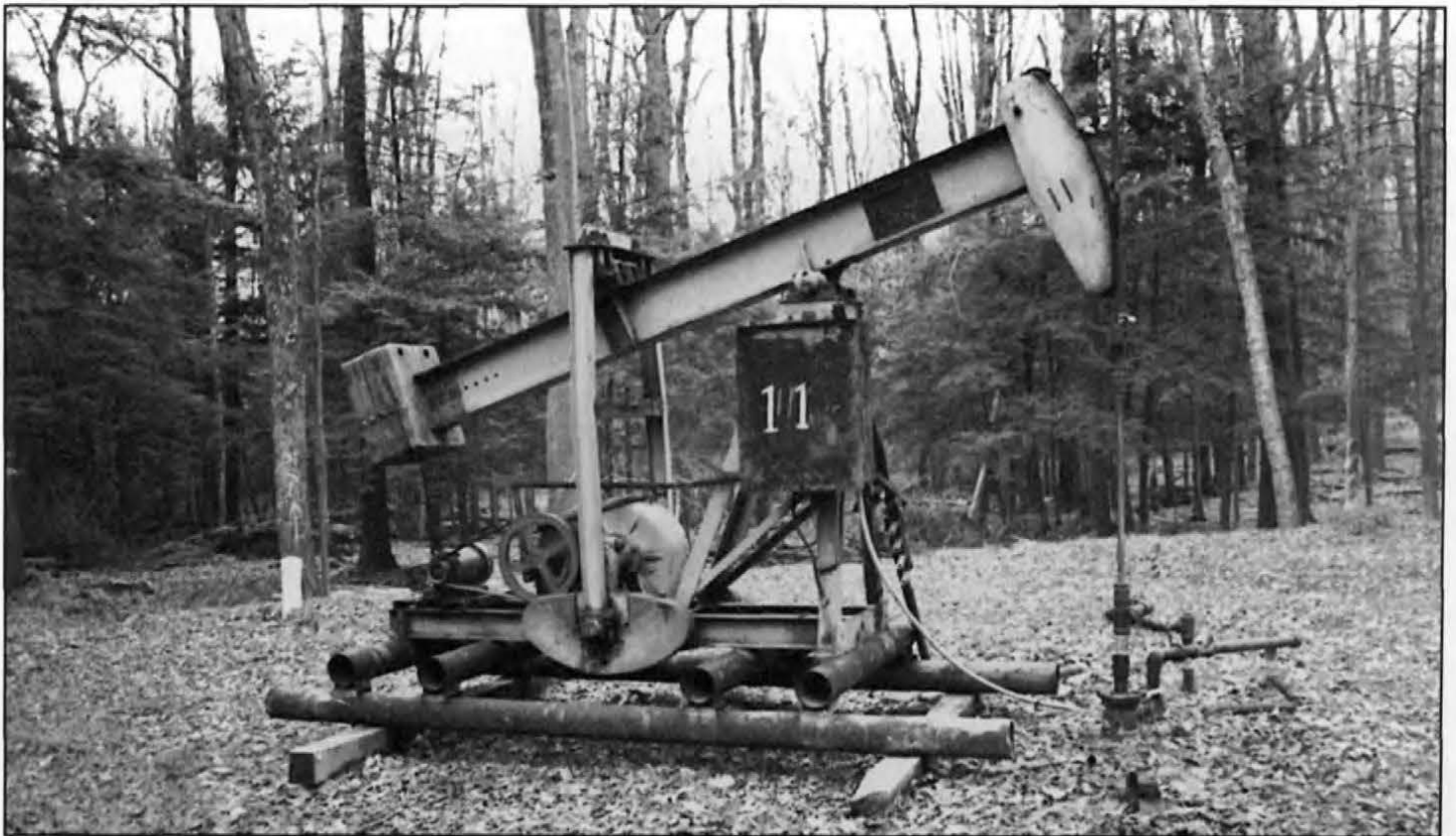
A unit pumping jack at Cooper Tract, 1994. This is the standard oil-lifting device today. Phil Ross
