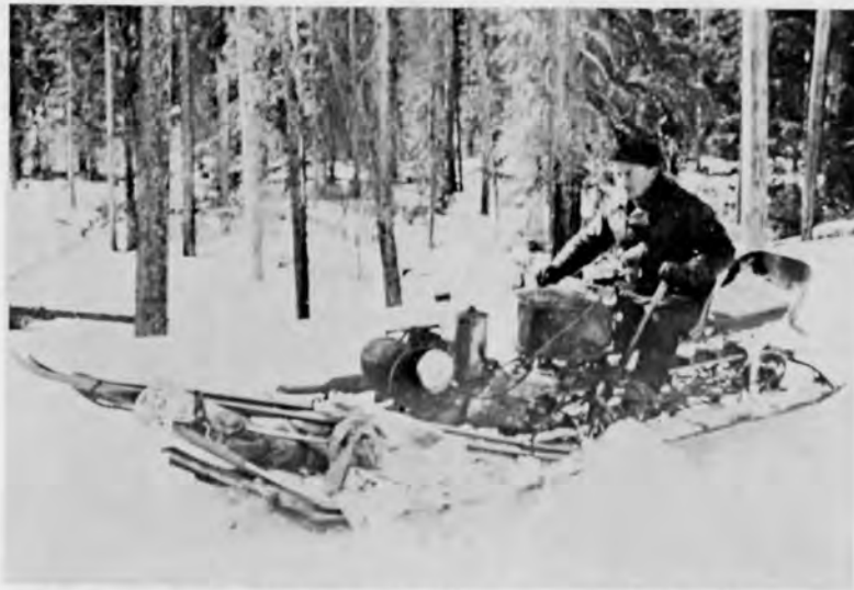
Snow machine built around "Indian motorcycle power plant.
