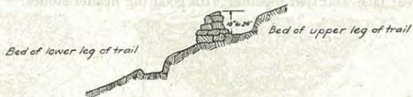
Fig. 15a Cross section 10' ahead of turn showing use of dirt rail or cut 18" to 24" deep and rocks on outer embankment to prevent cross cutting on switch back
