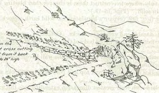
Fig. 15 Showing use of rock wall to prevent cross cutting at turns of switch backs. Use only where rock of substantial sizes are handy (Not needed on secondary trails).
