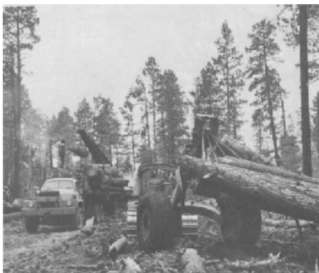
Figure 24. Caterpillar tractor and logging arch skidding ponderosa pine sawlogs to loading site, Apache National Forest, 1960.
