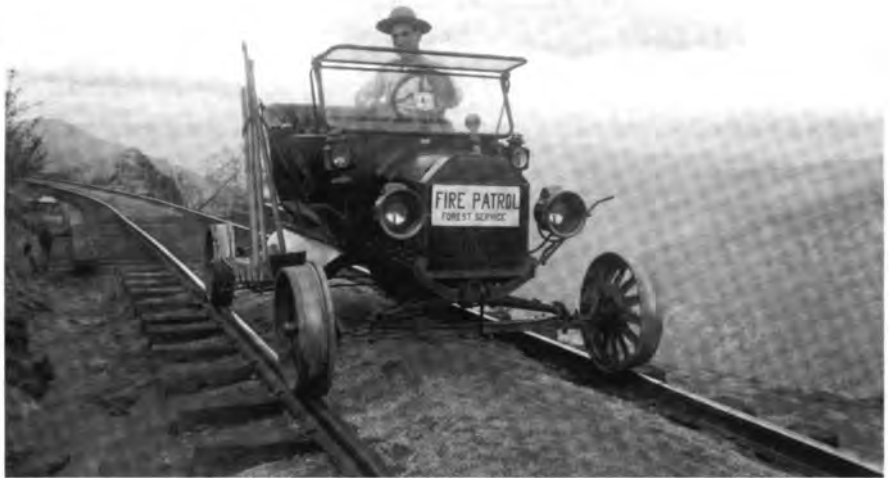
Ranger C. E. Jordan and Ford Roadster fitted with flanged wheels for use on San Joaquin and Eastern R. R. Sierra National Forest.
