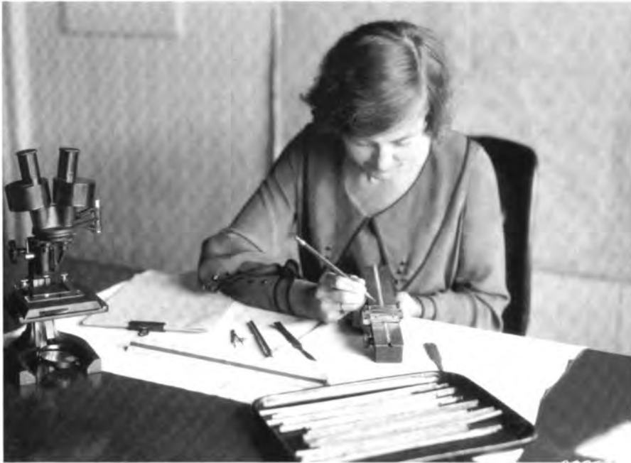
Reading the life history of trees and forests from the annual rings of increment cores taken from living trees. Instrument invented by Duncan Dunning of the California District, U.S. Forest Service. 1925
