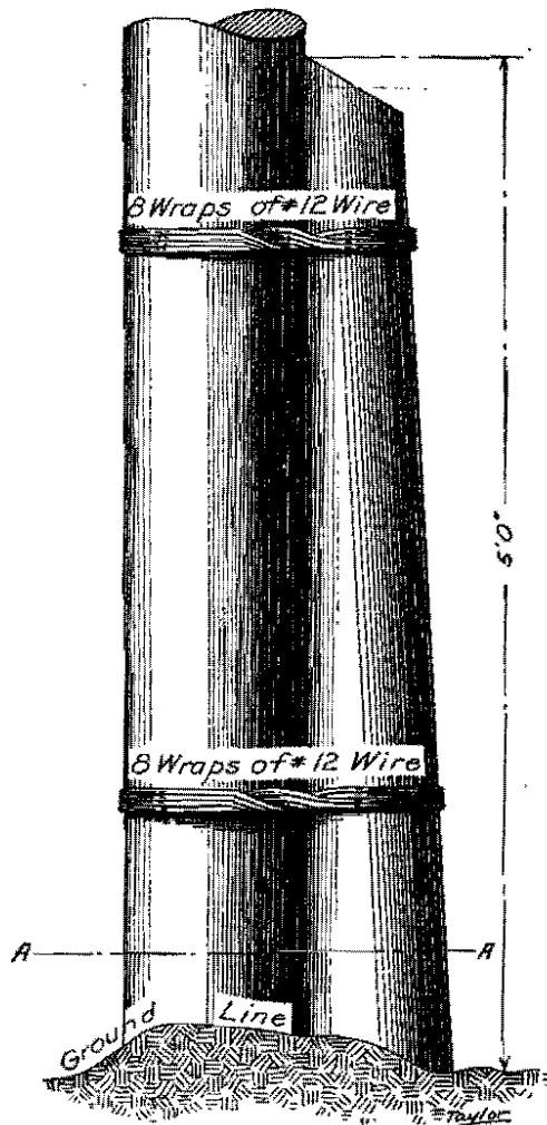
FIG. 30.—Reinforcement of stub of poles.
