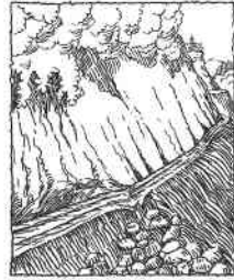
Dips help drain low service roads.
