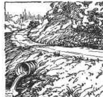
Culverts are necessary on in-sloped trails.
