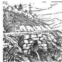
End wall for culvert.
