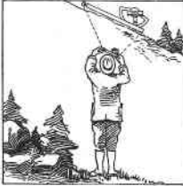
Measuring distant slope with Abney.
