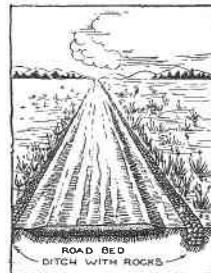
Intercepting ditches separate road bed from water source.
