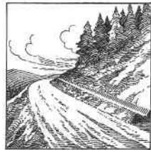
Intercepting ditches keep water off road (note cross-section).
