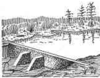
Concrete dam for water storage.
