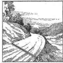
An open-top culvert.
