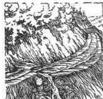
Water bars are used as temporary drainage structures.
