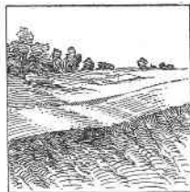
A break to carry water across trail.
