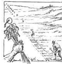
Use of pins in chaining.
