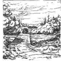
Low-water bridges are sloped—permitting high water to flow over the decking.
