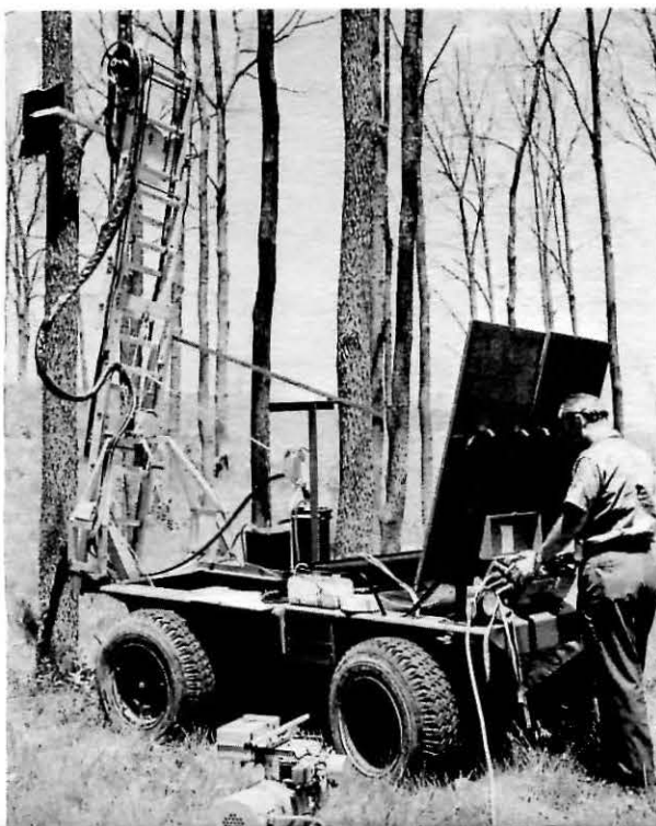
This mobile device was developed at the Delaware, Ohio, Laboratory for X-raying living trees as an aid to insect and disease research.
