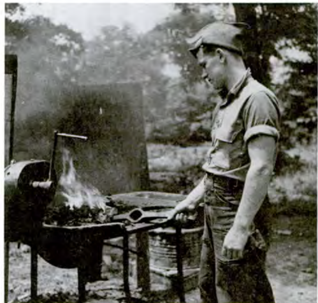
Figure 72.—A Civilian Conservation Corps enrollee tempering a pick head in an open forge at Lost Creek CCC Camp (F-26), near Norton, Va., in Clinch Ranger District, Jefferson National Forest, in June 1938. (NA:95G-367179)
