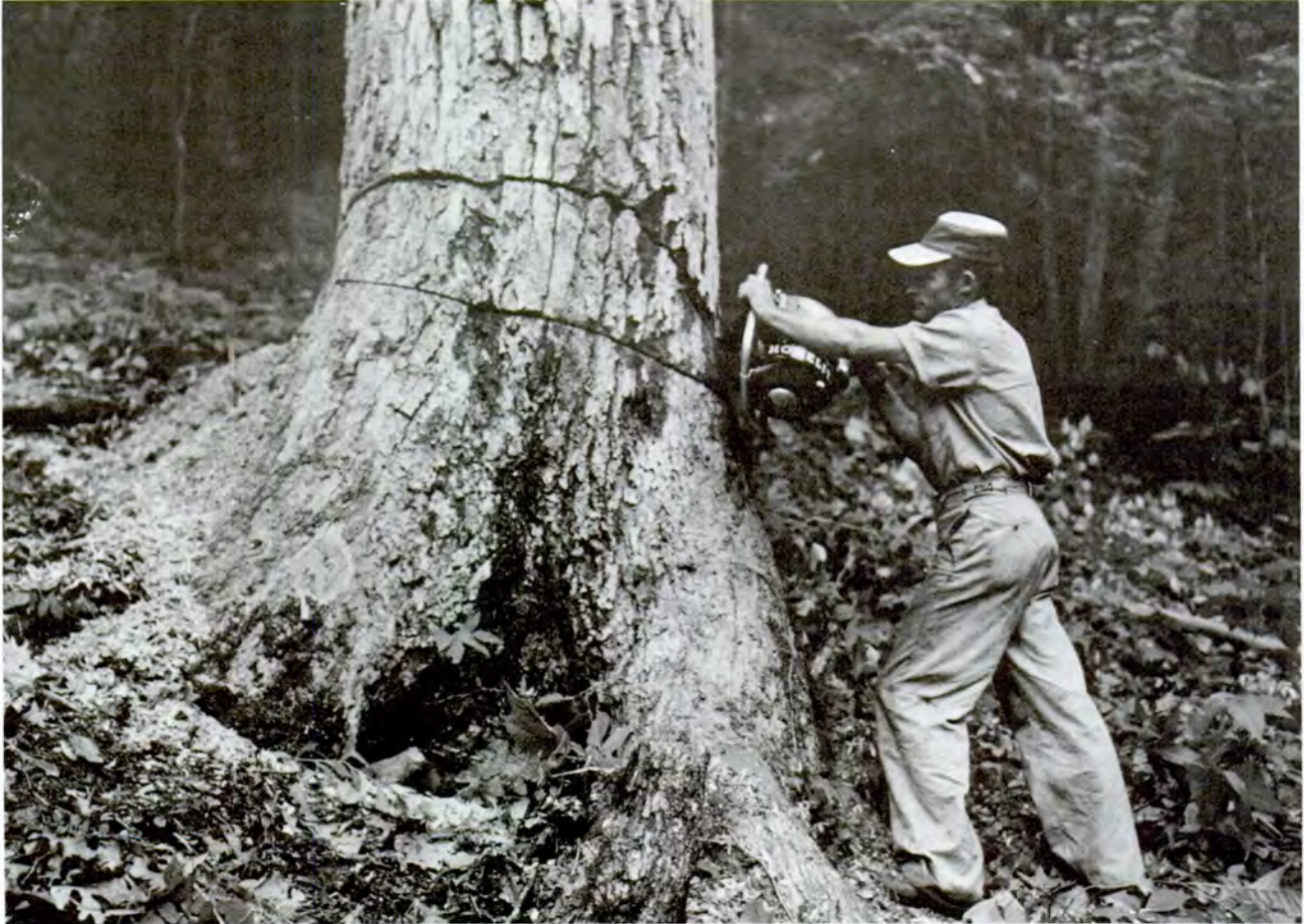
Figure 98.—Cutting a big notch in base of 38-inch mature yellow-poplar tree to fix direction of fall before felling, using one-man power chainsaw, on a timber sale in Chattahoochee National Forest, North Georgia, in October 1956. (Forest Service photo F-481523)
