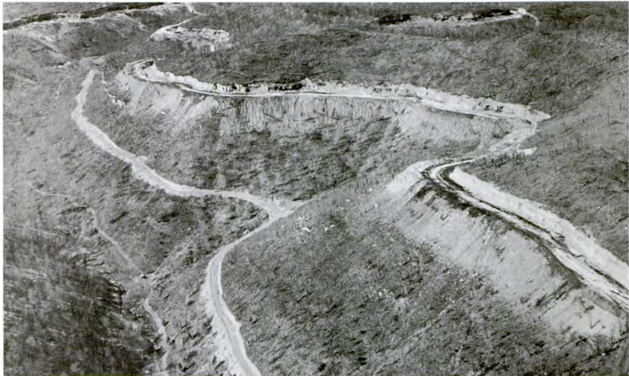
Figure 106.—Hillsides scarred by strip and auger coal mining along Beech Fork, Leslie County, Ky., in 1965. A common sight then in Redbird Purchase Unit. Acid soil debris leached down to pollute streams and kill fish for many years. New highway and old road cut slope at lower levels. (Forest Service photo F-512684)
