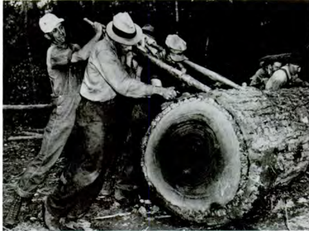
Figure 78.—Crew using peavies to roll a huge yellow-poplar log down to loading platform on Chattahoochee National Forest, July 1941. (Forest Service photo F-414105)
