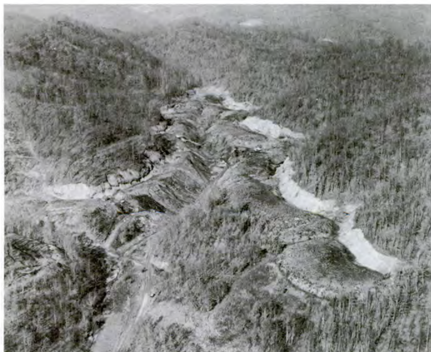
Figure 106.—Hillsides scarred by strip and auger coal mining along Beech Fork, Leslie County, Ky., in 1965. A common sight then in Redbird Purchase Unit. Acid soil debris leached down to pollute streams and kill fish for many years. New highway and old road cut slope at lower levels. (Forest Service photo F-512684)
