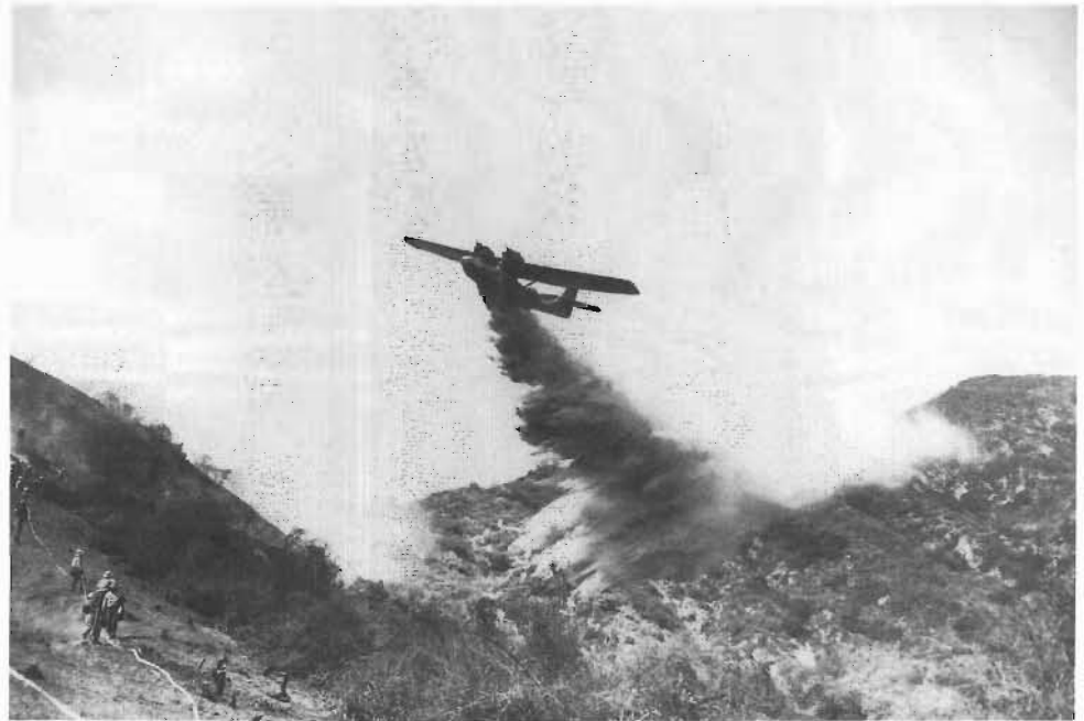
Air tanker dropping borate slurry at the head of the Monrovia fire, Angeles National Forest, California, October 1958.
