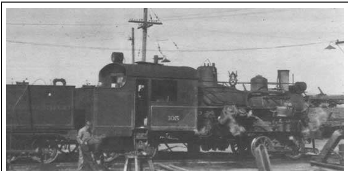
Figure 31. Santa Fe Northwestern locomotive Number 105 in the sawmill yards at Bernalillo, New Mexico circa 1933. This was the second Heisler geared locomotive on the railroad. It weighed about 60 tons, and all twelve wheels were driven by a line shaft centered under the locomotive. (Photo by Charlie Pratt)
