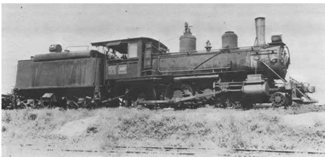
Figure 33. Number 107 of the Santa Fe Northwestern Railway at Bernalillo, New Mexico. By this time, the locomotive had been converted to oil fuel and an oil tank was installed in the former coal space of its tender. (Photo by Robert M. Hanft made July 31, 1939)
