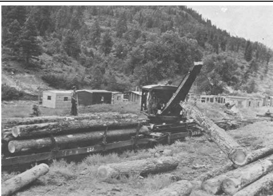
Figure 68. An American Hoist and Derrick diesel loader working at O'Neil Landing in the summer of 1939. The logs, of apparent 32-foot length, are being loaded on SFNW steel log cars. Typical portable living quarters may be seen beyond the cars. Once the local harvest was complete, these buildings could be hoisted aboard flat cars and taken to a new location. This portability is significant to archeologists who later find only a few foundation stones where once many men lived. (Photo by Yale Weinstein)
