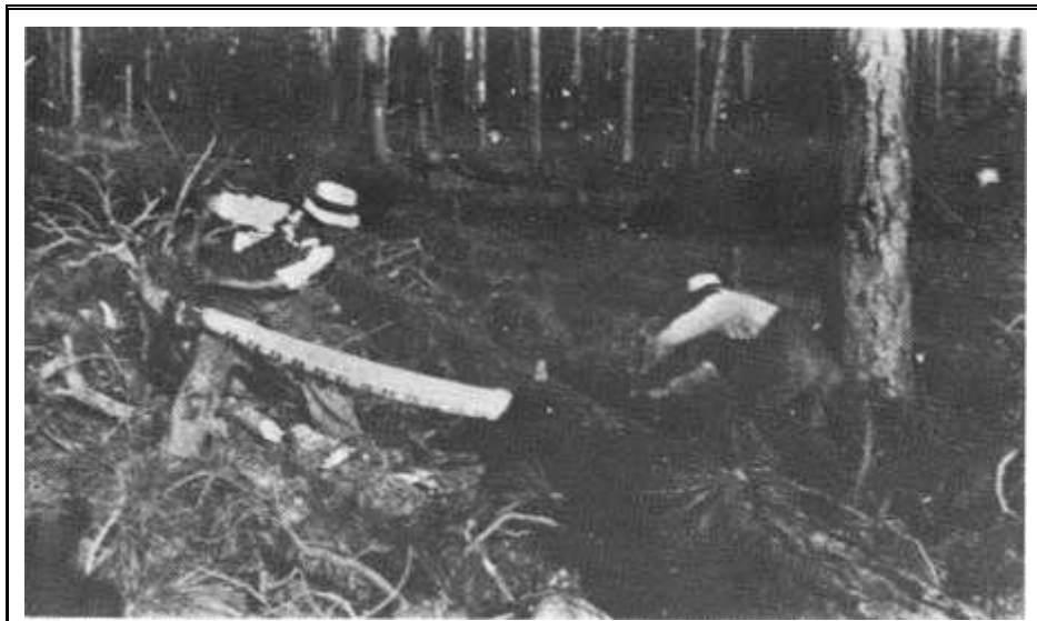
Figure 27. Bucking a felled tree into logs twenty-feet long for skidding, circa 1932. The chain saw had yet to make its appearance. (From the collection of T. P. Gallagher, Jr.)
