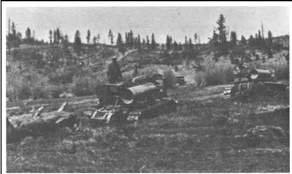
Figure 28. Two caterpillar tractors skidding a log across soft ground circa 1932. The railroad landing can be seen at the edge of the valley in the left background. (From the collection of T. P. Gallagher, Jr.)
