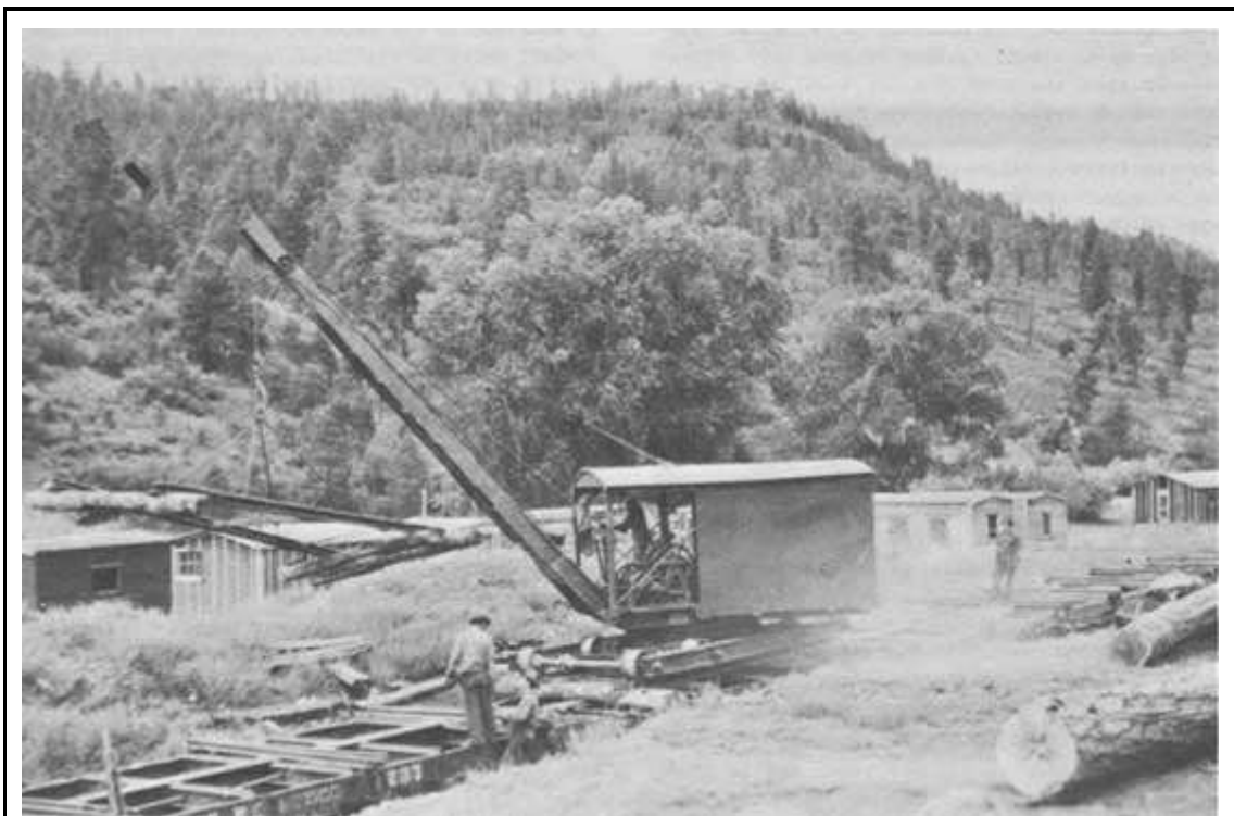
Figure 44. American Hoist and Derrick diesel loader at O'Neil Landing in the summer of 1939. The loader is moving a set of rails into position on the next log car in preparation for its movement to that car. The long carriage of the loader with its wheels can be clearly seen. The log car on the left is one of a group of old steel cars purchased in 1930 from the Ferrocarril Nor Oeste de Mexico. (Photo by Yale Weinstein)
