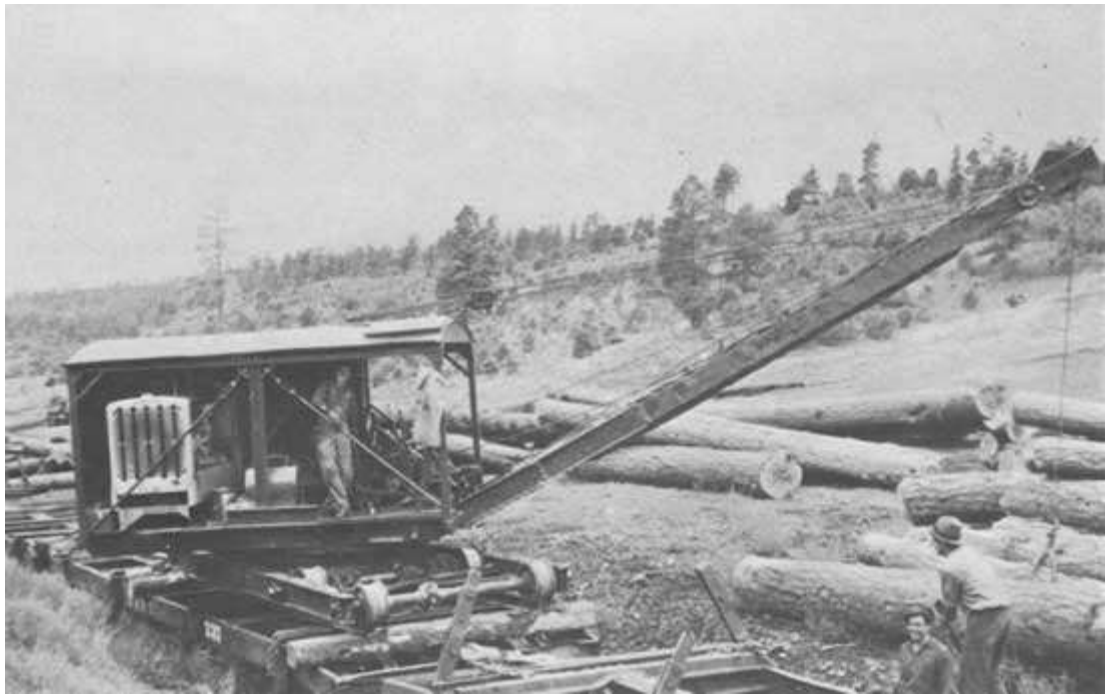
Figure 90. An American Hoist and Derrick loader at O'Neil Landing in the summer of 1939. The steam-to-diesel conversion is evident. The steam boiler, cylinders, and water tank were removed and replaced by a diesel engine and power take-off mounted on a slide-in frame, Will Everett is the loaderman. (Photo by Yale Weinstein)
