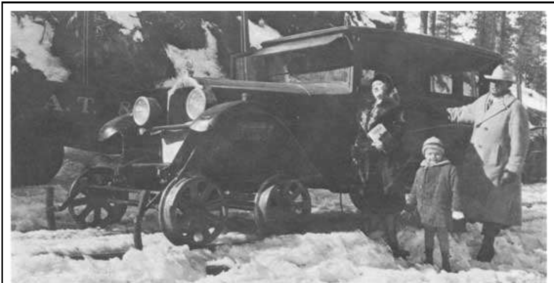
Figure 24. One of the more elaborate rail-autos, probably at Porter circa 1932. This four-door sedan was modified with a light four-wheel truck in place of the front wheels and steering gear, and stamped-steel railroad wheels on the rear axle. The ride was hard, but the convenience of such a vehicle was a necessity during the winter months when snow and mud blocked what few roads there were. ( T. P. Gallagher, Jr., collection )
