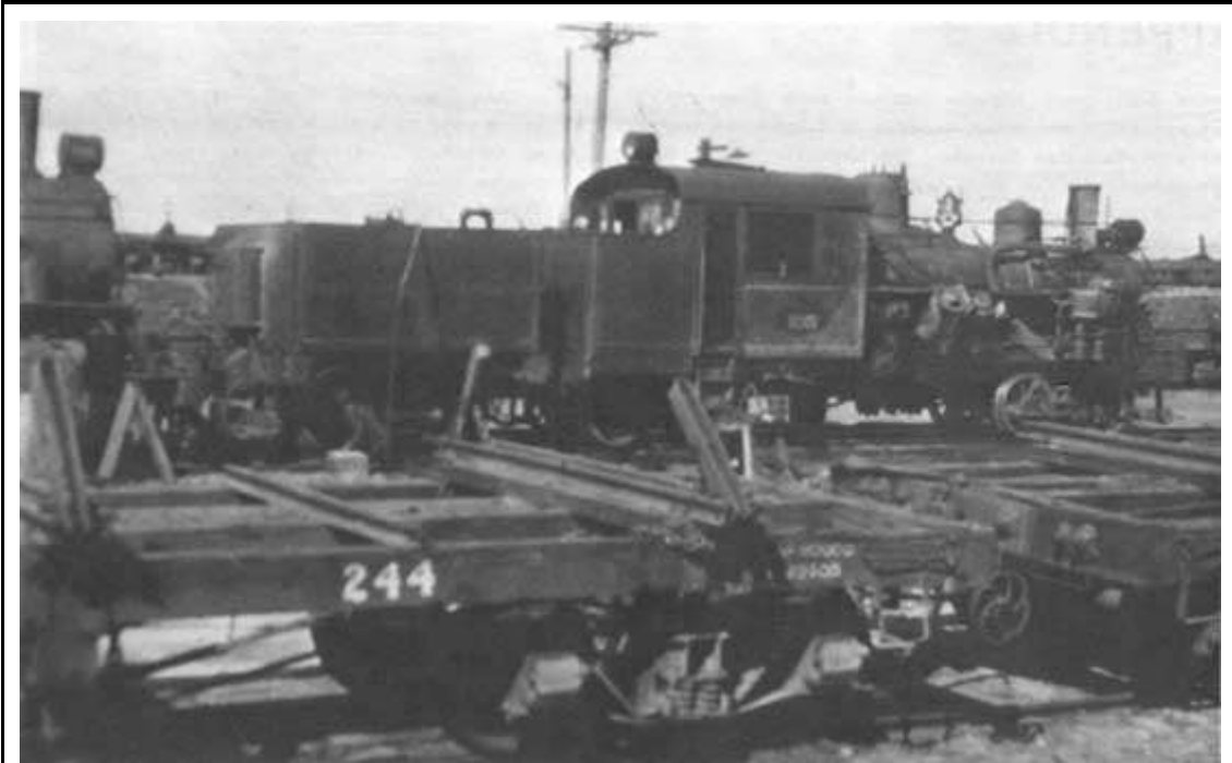
Figure 67. A 3T Heisler, locomotive Number 105, of the Santa Fe Northwestern Railway at Bernalillo, circa 1933. Log car Number 244 shows its open-frame construction and folding-stake log bunks. (Photo by Charlie Pratt)
