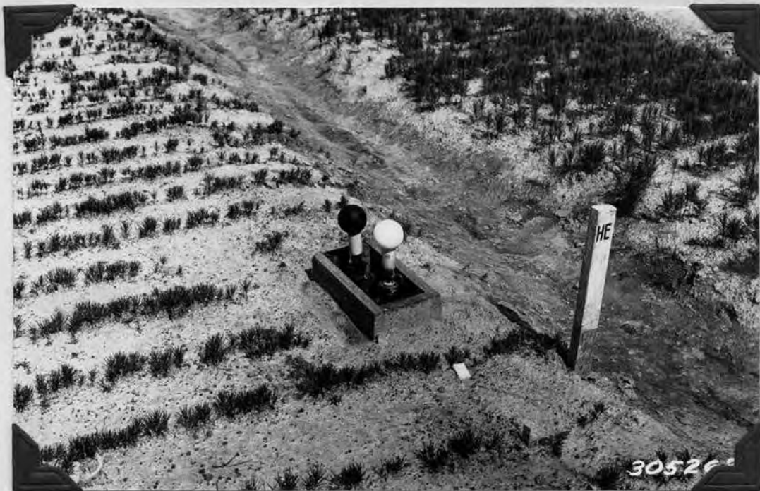
Black and white porous clay cup anemometers to measure evaporation.
