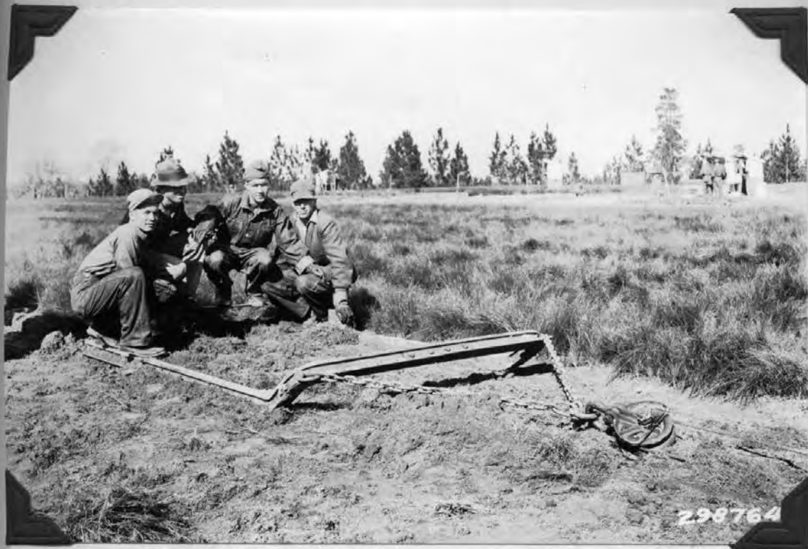
A closer view of the tree lifter just after it has been drawn through a bed of longleaf
