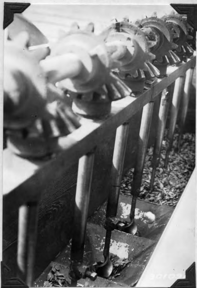
Interior view of seedbox of the Williamson longleaf drill seeder.
