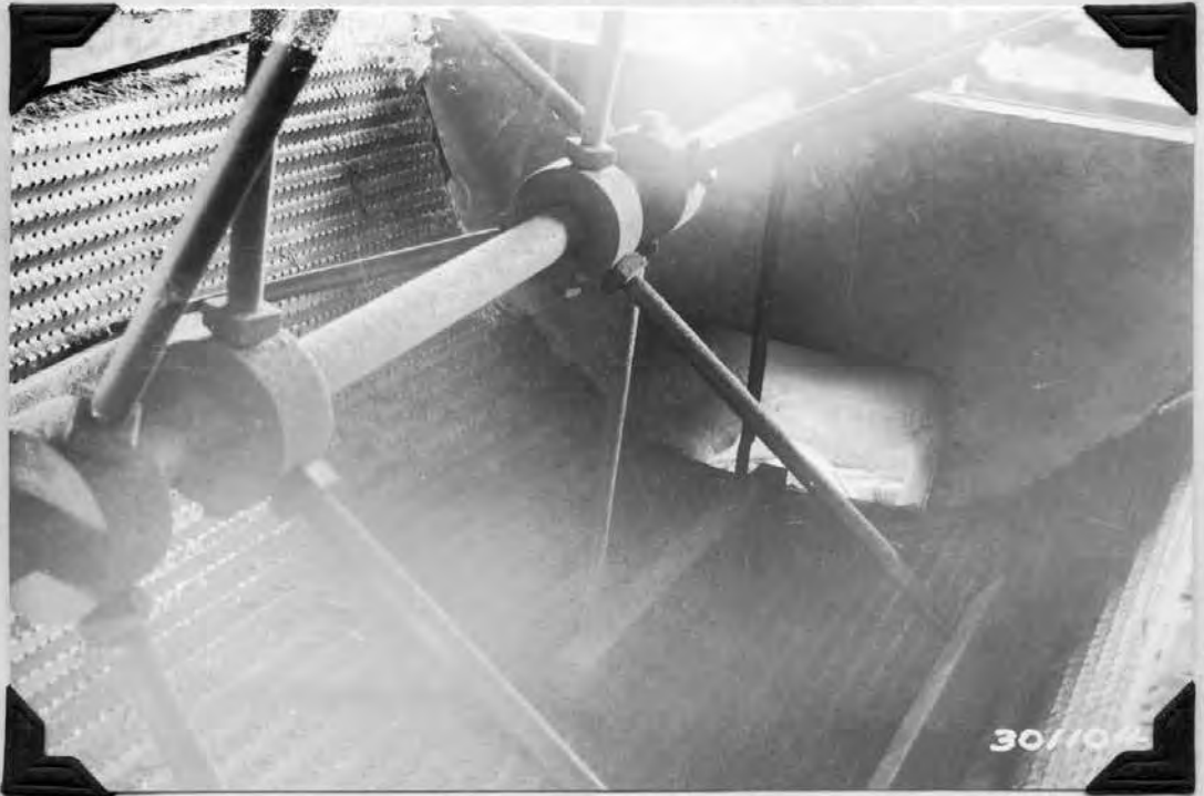
Interior of dewinger, showing perforated, corrugated surface, and bristle-brushes. Chute at lower end.
