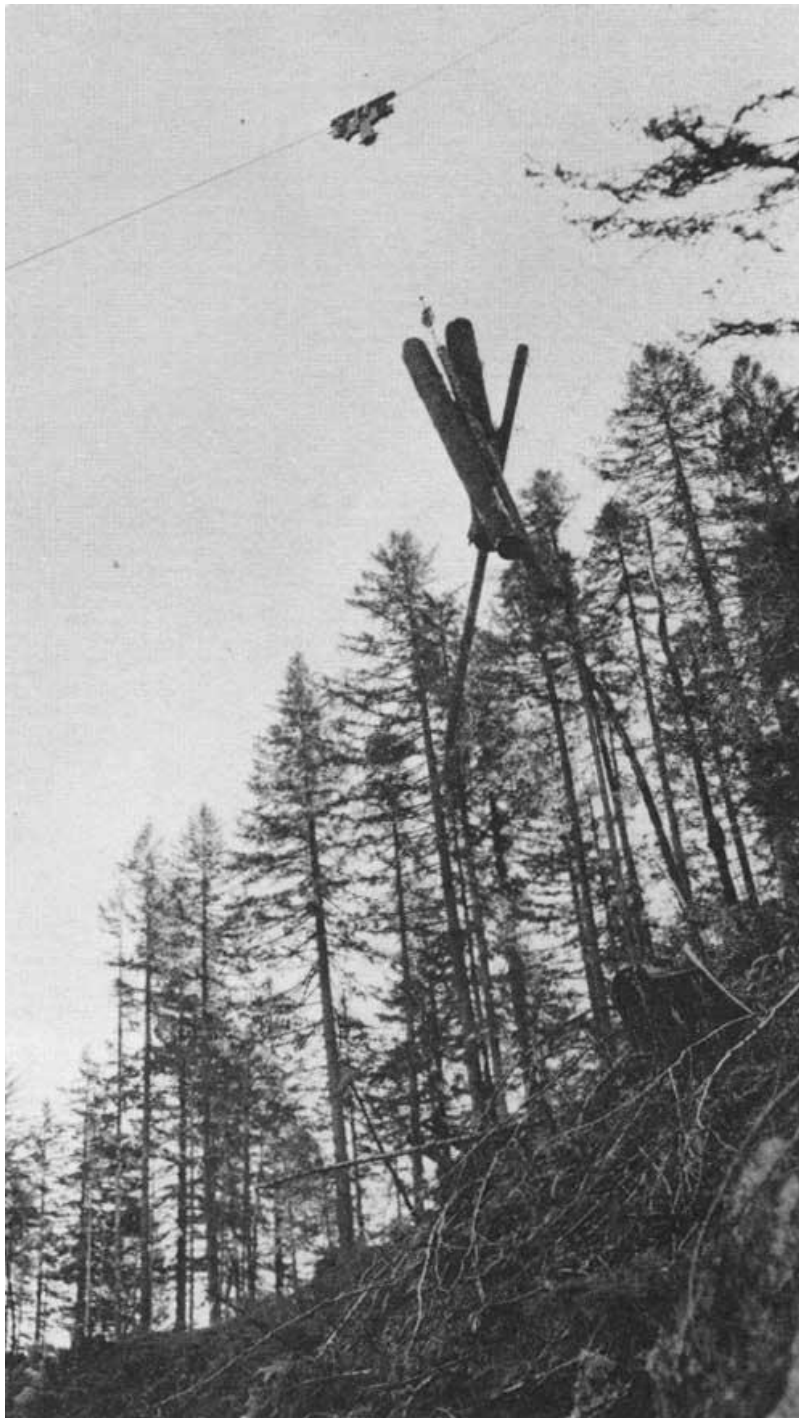
Wyssen Skyline Crane - logs being lifted to the carriage in the H.J. Andrews Experimental Forest, c. 1970.
